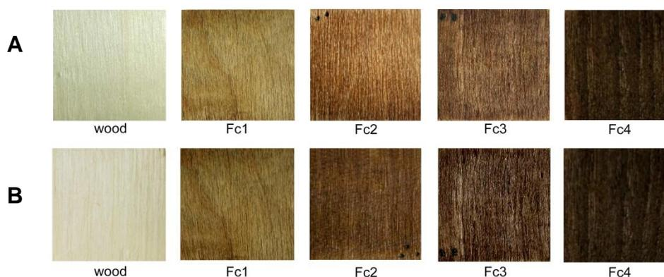
**Fig. 7.** (A) Color and (B) photochromism of non-modified and  $\text{WO}_3$ -modified wood samples
