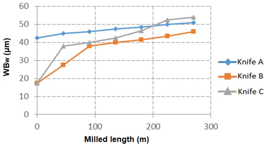
**Fig. 12.** Dependence of cutting wedge wear on milled length;  $5000 \text{ min}^{-1}$ ;  $a_e = 1 \text{ mm}$ ;  $v_f = 6 \text{ m/min}$ ,  $8 \text{ m/min}$ ,  $10 \text{ m/min}$ ,  $12 \text{ m/min}$ , and  $14 \text{ m/min}$
