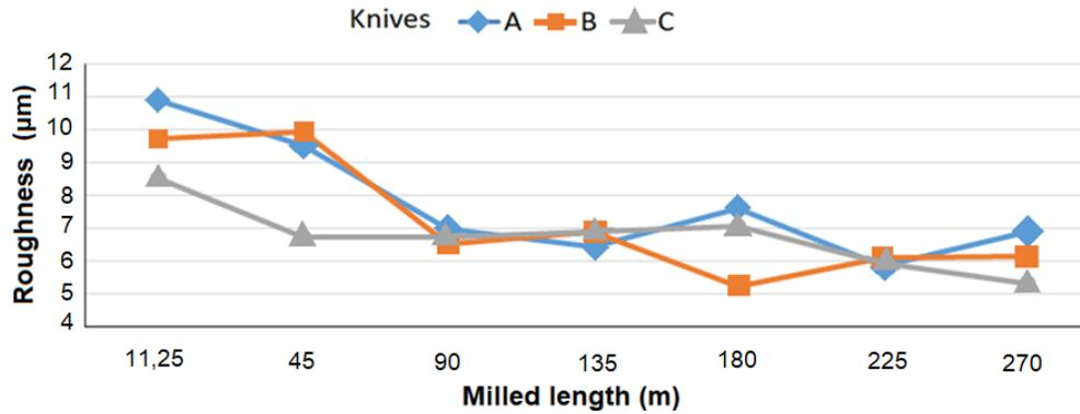
**Fig. 11.** Effect of milled length on the surface roughness  $R_a$ ;  $5000 \text{ min}^{-1}$ ;  $a_e = 1 \text{ mm}$ ;  $v_f = 6 \text{ m/min}$ ,  $8 \text{ m/min}$ ,  $10 \text{ m/min}$ ,  $12 \text{ m/min}$ , and  $14 \text{ m/min}$
