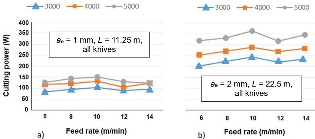
**Fig. 9.** Effect of cutting depth and feed rate on cutting power: (a)  $a_e = 1 \text{ mm}$ ,  $L = 11.25 \text{ m}$ , all knives; (b)  $a_e = 2 \text{ mm}$ ,  $L = 22.5 \text{ m}$ , all knives
