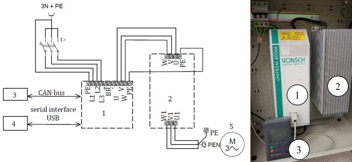
**Fig. 4.** Connection of devices for power measurement: (1) frequency converter (UNIFREM 400 007 M, VONSCH, Brezno, Slovakia), (2) sinusoidal filter (SKY3FSM25, VONSCH, Brezno, Slovakia), (3) operating panel, (4) laptop, (5) 3-phase asynchronous motor (2.2 kW, 2880 min<sup>-1</sup>)
