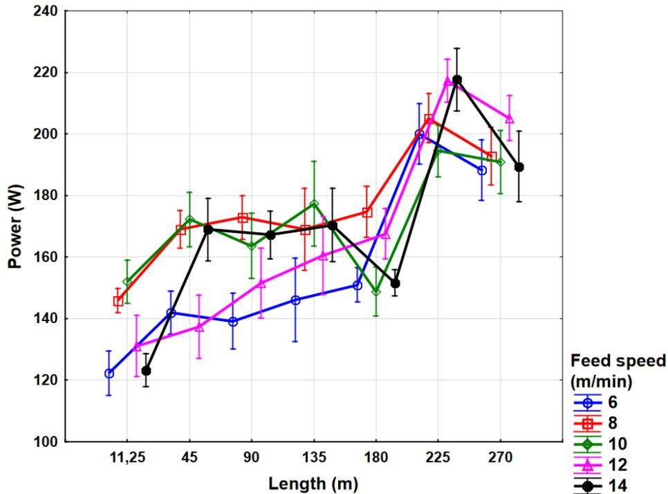
**Fig. 8.** Weighted means of power depending on milled length at different feed rates for all knives; 5000  $\text{min}^{-1}$ ;  $a_e = 1 \text{ mm}$
