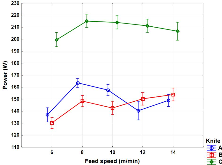
**Fig. 7.** Weighted means of cutting power for all knives; 5000  $\text{min}^{-1}$ ; cutting depth  $a_e = 1$  mm; milling length  $L = 11.25$  m to 270 m
