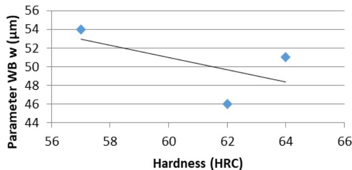
**Fig. 13.** Relation between the hardness and wear parameter;  $5000 \text{ min}^{-1}$ ;  $a_e = 1 \text{ mm}$ ;  $v_f = 6 \text{ m/min}$ ,  $8 \text{ m/min}$ ,  $10 \text{ m/min}$ ,  $12 \text{ m/min}$ , and  $14 \text{ m/min}$
