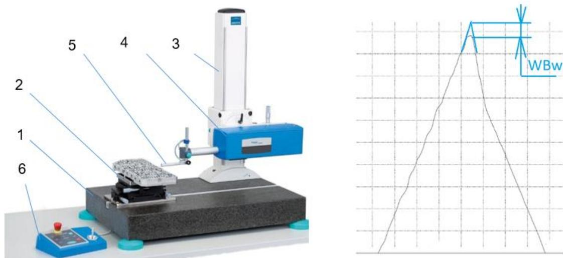
**Fig. 6.** Contour measuring system:  $WB_w$  – displacement of cutting edge along the axis of cutting wedge angle  $\beta$  (Porankiewicz *et al.* 2005), (1) granite foundation slab, (2) table, (3) console, (4) arm, (5) contact head, (6) controlling desk
