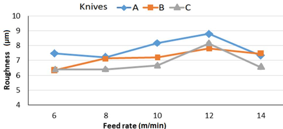
**Fig. 10.** Effect of feed rate on the surface roughness; 5000  $\text{min}^{-1}$ ;  $a_e = 1$  mm; milling length  $L = 11.25$  m to 270 m
