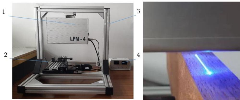
**Fig. 5.** Assembly of laser profilometer: (1) profilometer head, (2) shift system for X-Z plane, (3) framework, (4) shift control unit
