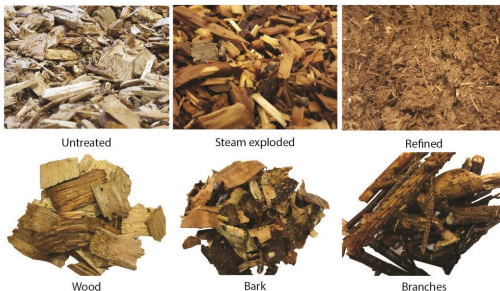
Fig. 1. The material analyzed: untreated, steam exploded, and refined forest residues and the separated fractions: wood chips, bark, and branches.
