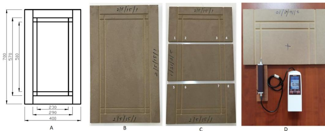
**Fig. 2.** Dimensions of pattern (A), test sample (B), measurement points (C), roughness tester (D)
