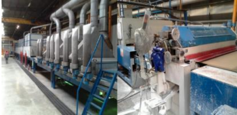
Fig. 3. Roller coater system used to coat panels
