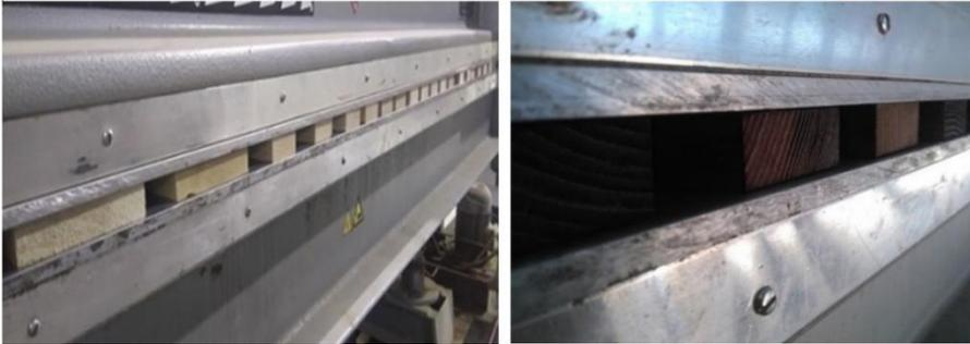
**Fig. 3.** Cooling the samples under pressure after TVM density operation
