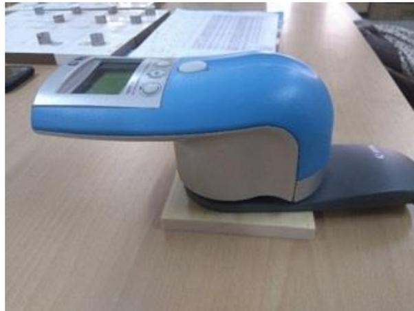
**Fig. 5.** Gloss measurement device
