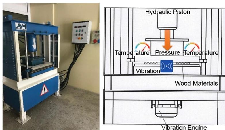
Fig. 2. TVM density press and working principle (Şenol 2018)
