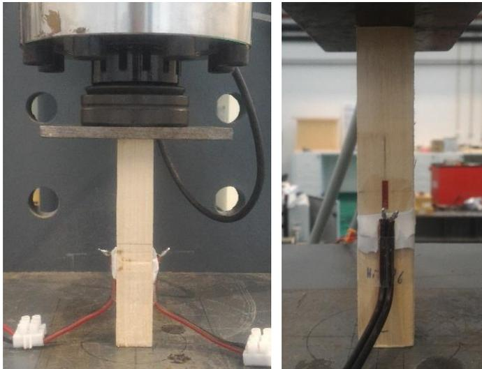
**Fig. 2.** Instrumented clear wood specimen for testing under compression parallel to the grain
