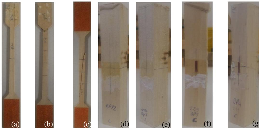
**Fig. 4.** Failure modes of specimens subjected to tension ((a), (b), and (c)) and compression ((d), (e), (f), and (g)) in parallel-to-grain tests
