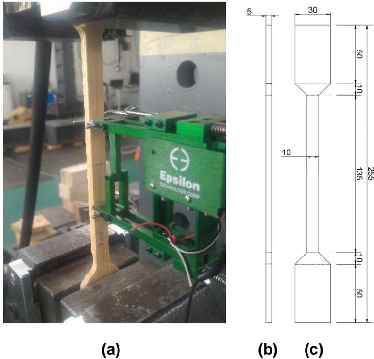
**Fig. 1.** Clear wood specimen instrumented for testing under tension parallel to the grain (a) and its nominal dimensions (mm): side view (b) and plan view (c)
