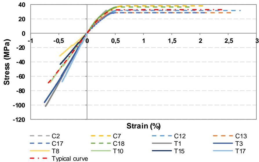
**Fig. 3.** Stress-strain representative curves obtained from experimental tension and compression tests parallel to the grain
