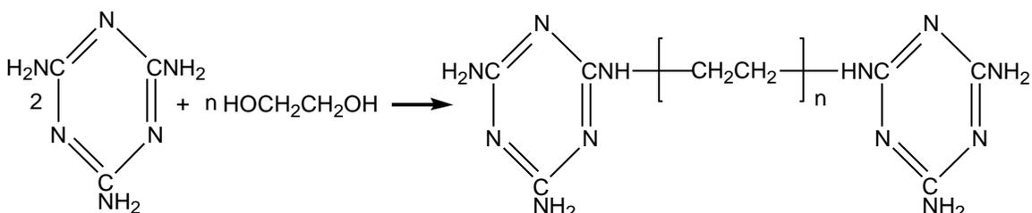
**Fig. 3.** Condensation reaction of ethylene glycol with melamine
