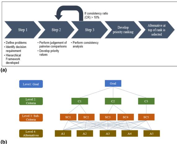
Fig. 1. (a) The AHP procedure; (b) The AHP hierarchy structure (Sapuan et al. 2011; Al-Ogla et al. 2016)
