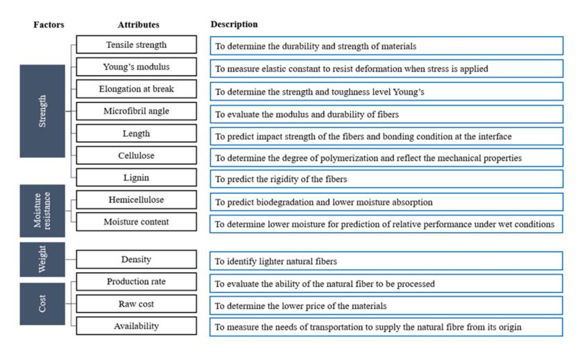
Fig. 2. Selection factors and attributes developed to find the most suitable natural fiber in biocomposites for food packaging application (Al-Oqla and Salit 2017; Mastura *et al.* 2017)
