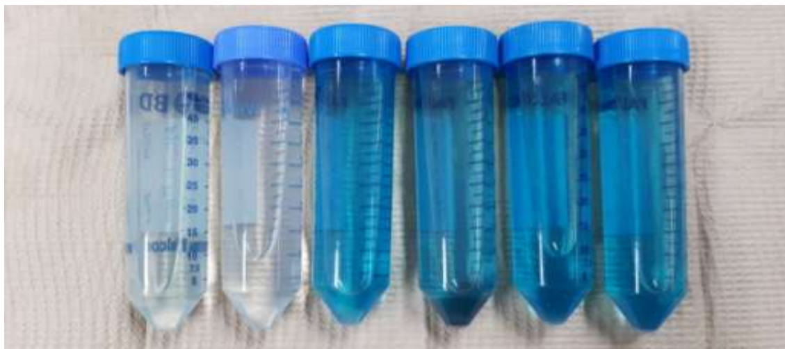
Fig. 7. Filtered 100 mL concentration methylene blue (MB) aqueous solution with different adsorbent samples (From left: S-C, S-2, S-4, S-6, S-8, and S-10)
