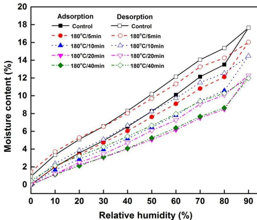
Fig. 7. Moisture adsorption and desorption behavior of kenaf fibers
