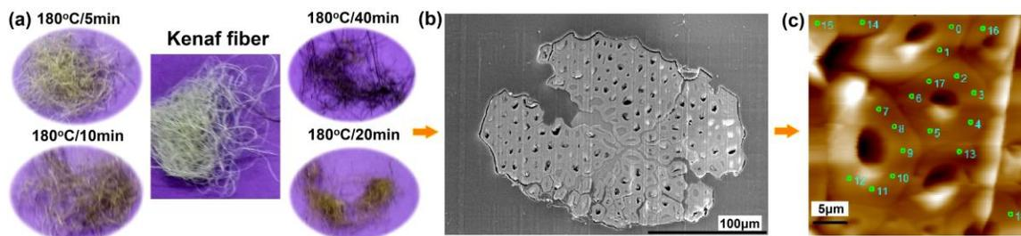
**Fig. 1.** Kenaf fiber sample preparation for NI test: (a) morphology photographs of kenaf samples; (b) kenaf fiber embedded in polypropylene; (c) NI test locations
