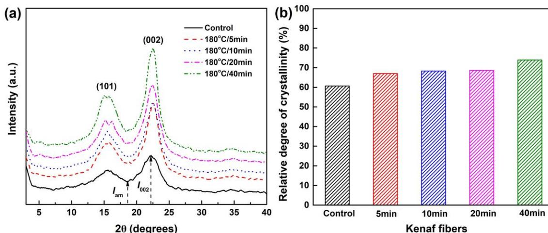
Fig. 5. XRD spectra of the control and treated kenaf fibers
