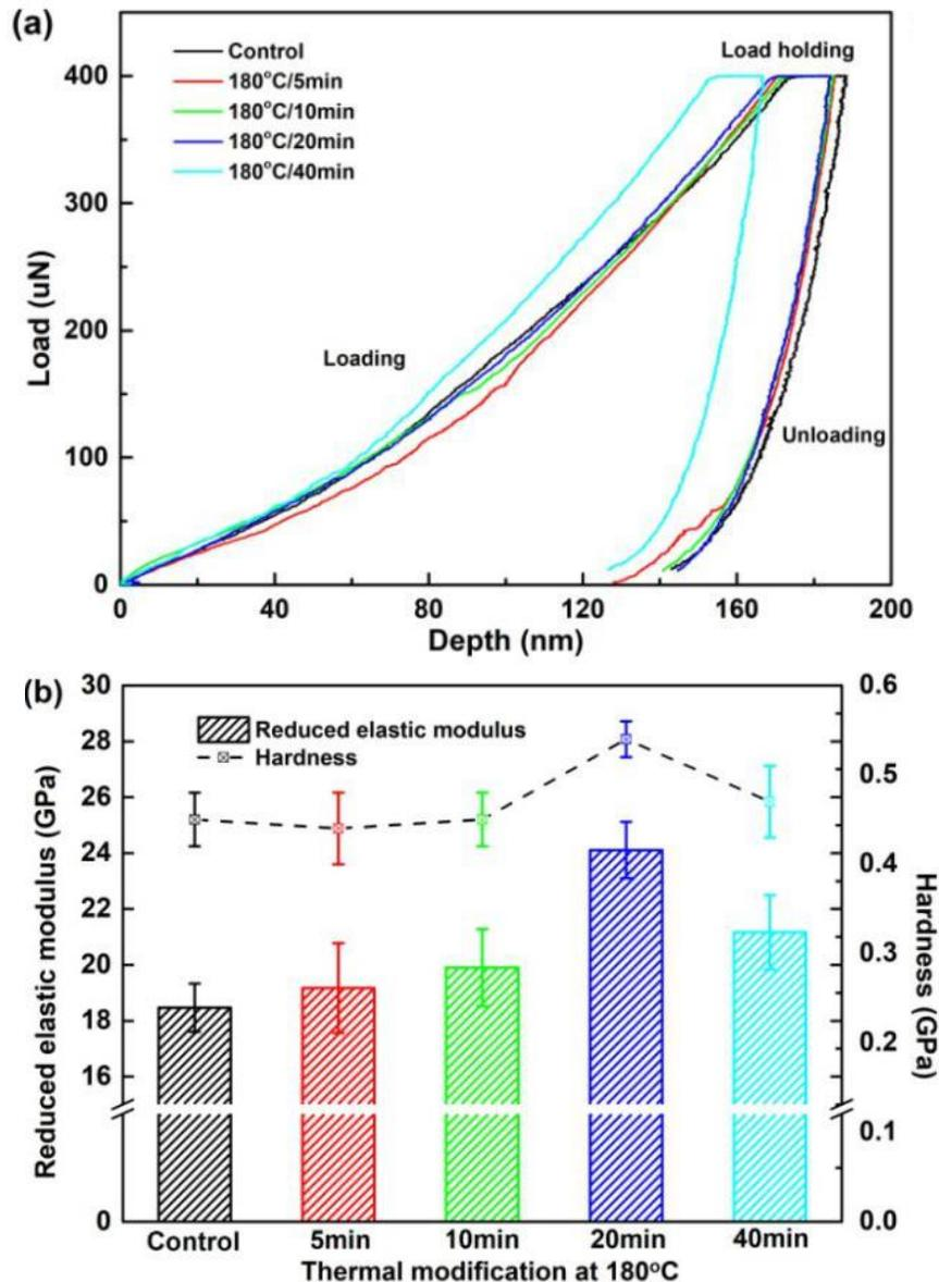
**Fig. 6.** Cell wall mechanics analysis by nanoindentation. (a) Typical indentation load-depth curves of cell walls; (b) reduced elastic modulus and hardness of kenaf fibers
