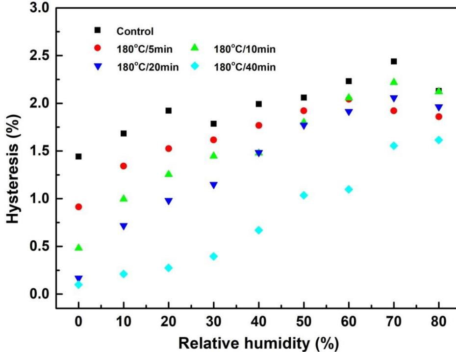
Fig. 9. Hysteresis of the control and treated kenaf fibers during the sorption process
