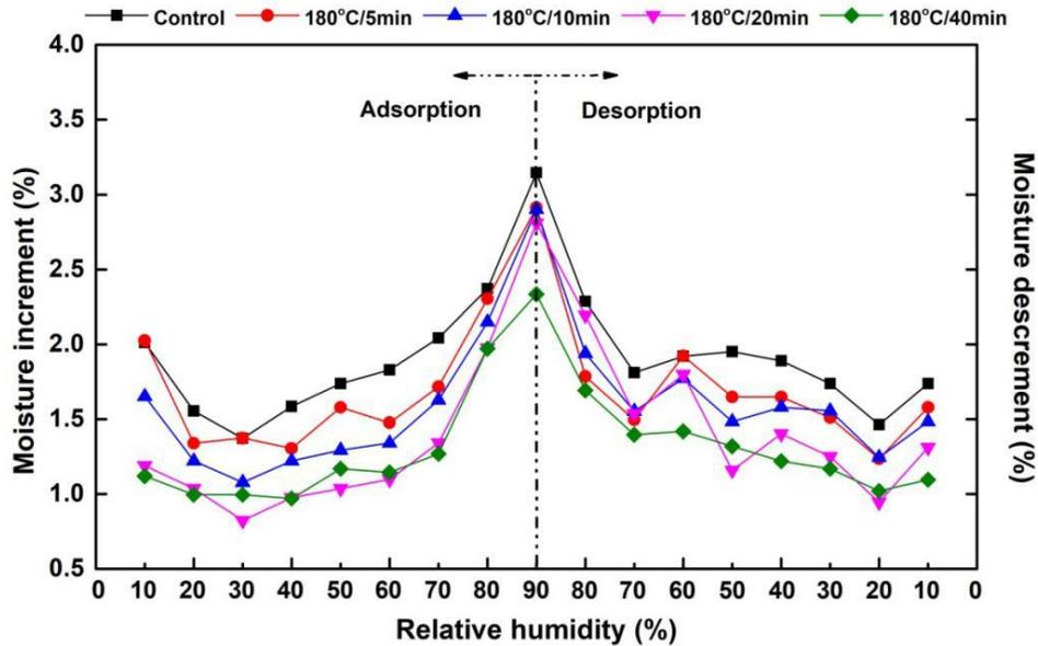
Fig. 8. Moisture content increment and decrement of kenaf fibers at given RH step.
