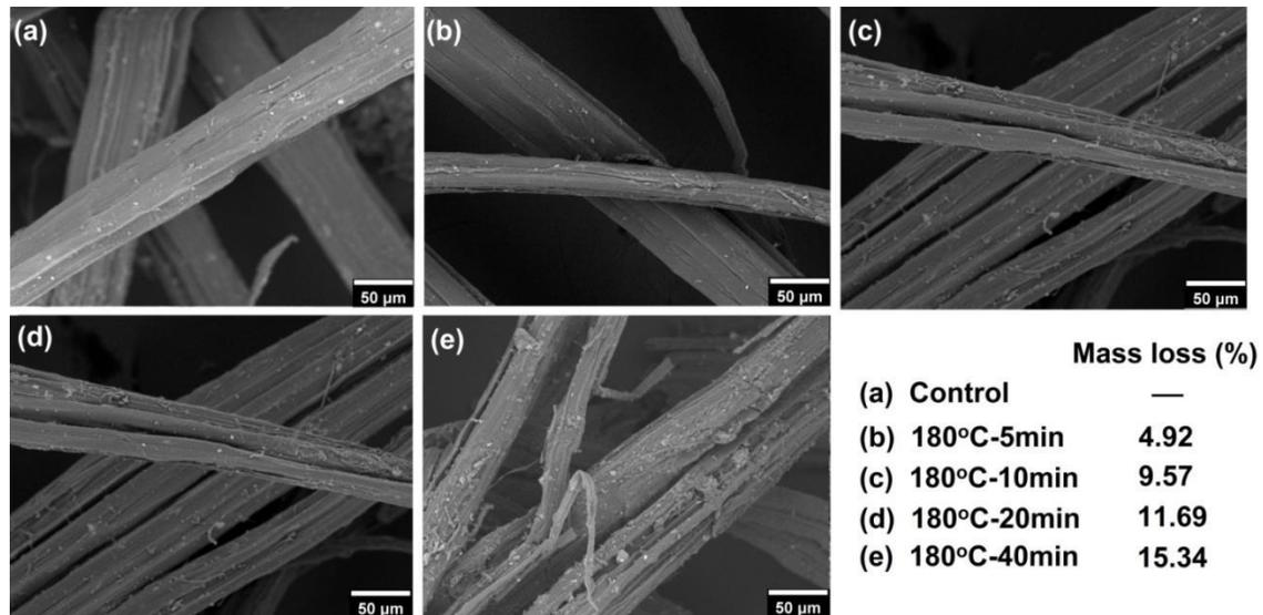
Fig. 3. Mass loss and morphology photographs of the control and treated kenaf fibers
