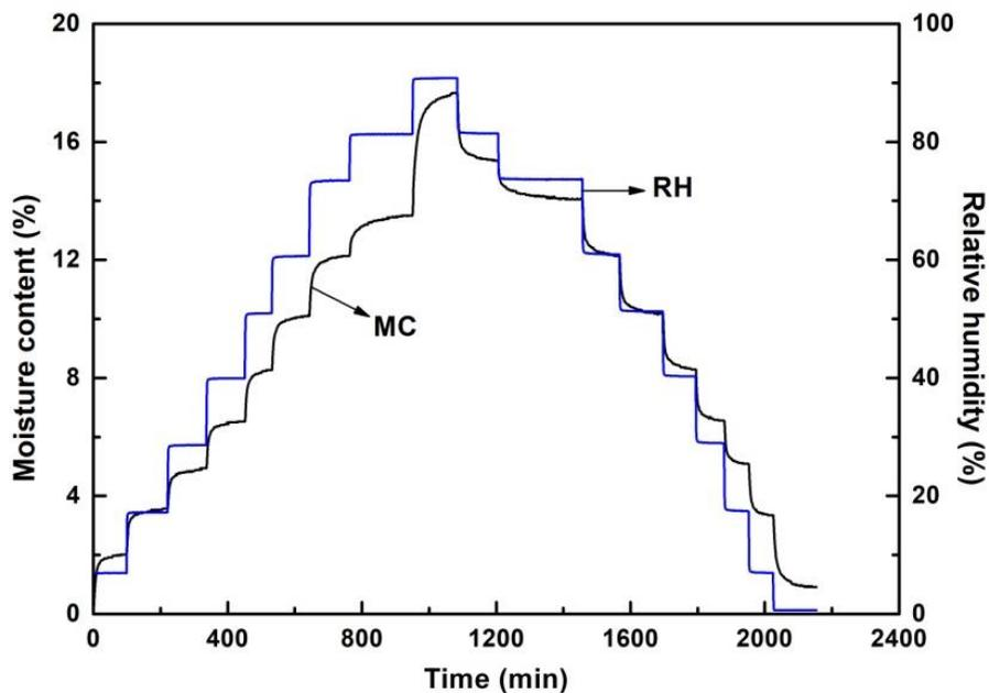
Fig. 2. Plot showing data from a typical DVS isotherm run for kenaf fiber
