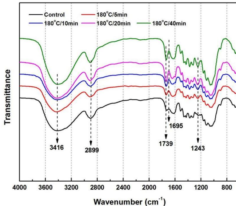
Fig. 4. FTIR spectra of the control and treated kenaf fibers
