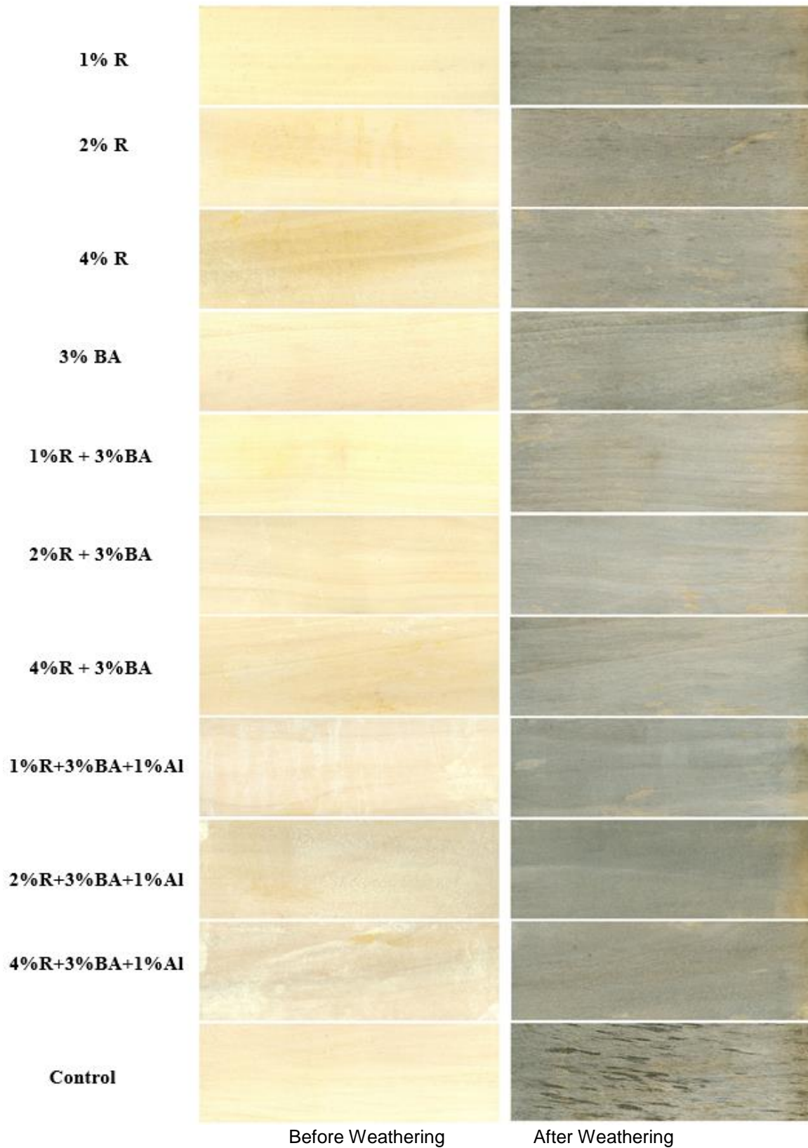
Fig. 3. Photographs of poplar wood samples before and after 3 months of natural weathering
