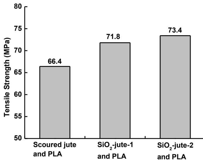
**Fig. 2.** Effect of modification method on the tensile strength of composites
