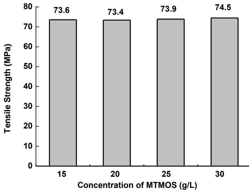
**Fig. 4.** Effect of MTMOS concentration on tensile strength of composites
