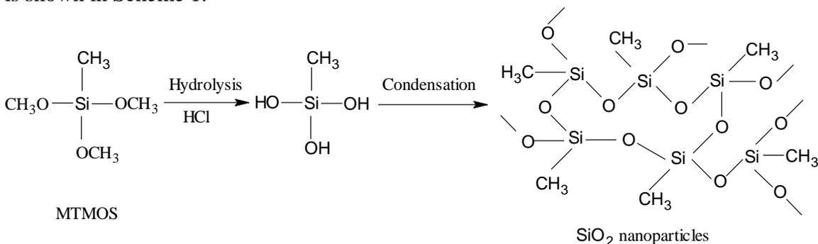
**Scheme 1.** Preparation of  $\text{SiO}_2$  nanoparticles hydrosol with MTMOS
