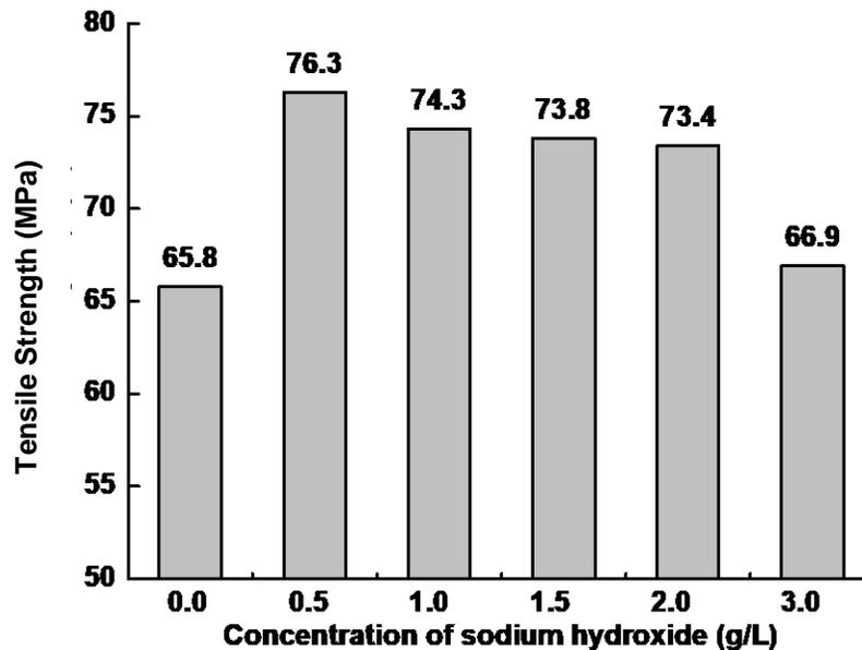
**Fig. 3.** Effect of NaOH concentration on the tensile strength of composites
