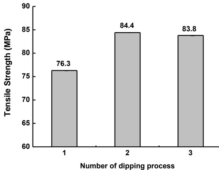
**Fig. 5.** Effect of number of dipping steps on tensile strength of composites
