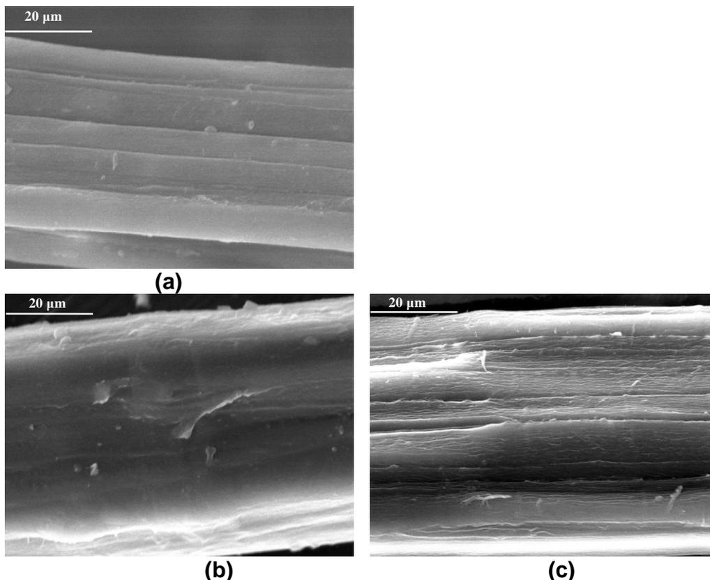
Fig. 1. SEM photographs of jute fibers: (a) scoured jute, (b) SiO<sub>2</sub>-jute-1, and (c) SiO<sub>2</sub>-jute-1
