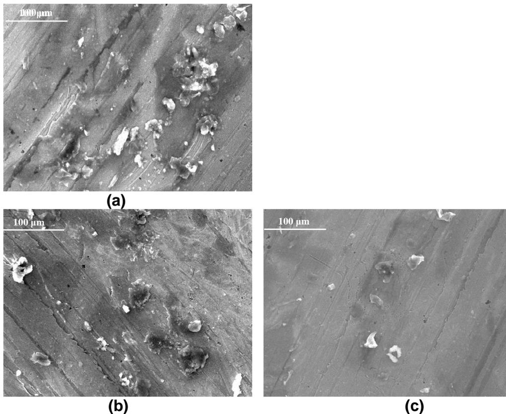
**Fig. 6.** Morphologies of fractured surface of composites: (a) scoured jute and PLA, (b) SiO<sub>2</sub>-jute-1 and PLA, and (c) SiO<sub>2</sub>-jute-2 and PLA
