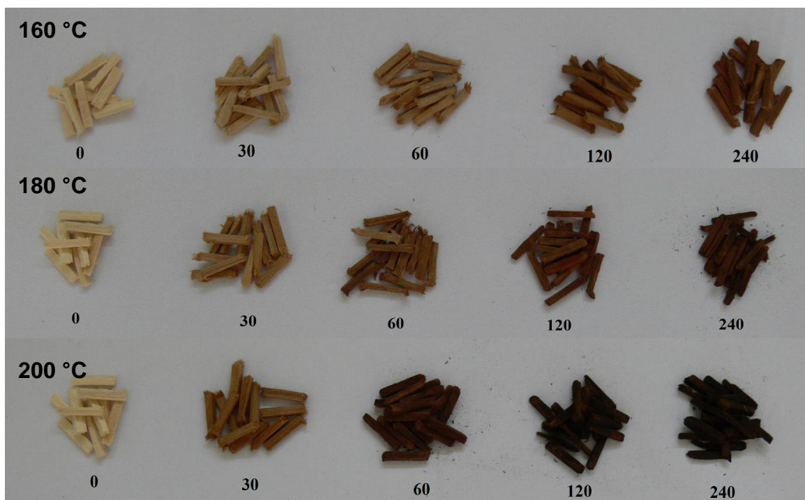
Fig. 1. Influence of pretreatment temperature and time on the colour of willow
