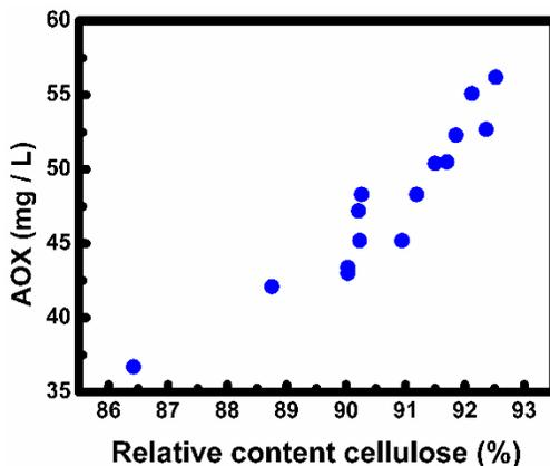
Fig. 6. Correlation between pulp relative cellulose content and wastewater AOX content
