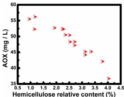
**Fig. 5.** Correlation between pulp relative hemicellulose content and wastewater AOX content
