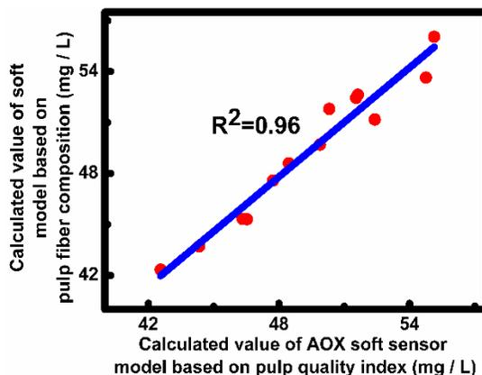
**Fig. 12.** Correlation between the calculated value of AOX with the soft sensor model based on pulp quality indices and calculated value of AOX with the model based on pulp fiber composition
