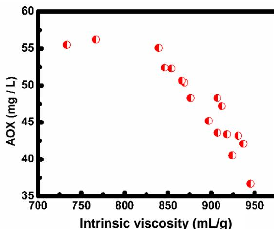
**Fig. 4.** Relationship between intrinsic pulp viscosity and wastewater AOX content
