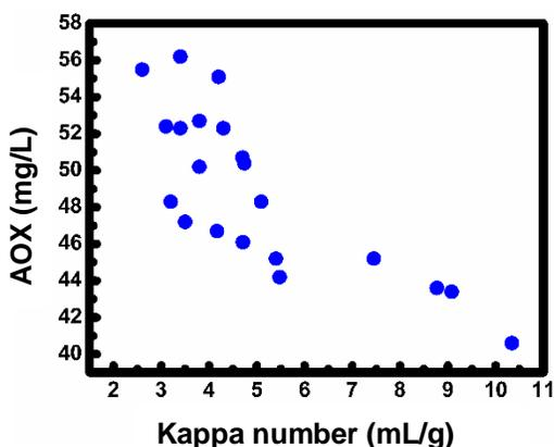
**Fig. 8.** Relationship between pulp Kappa number and wastewater AOX content
