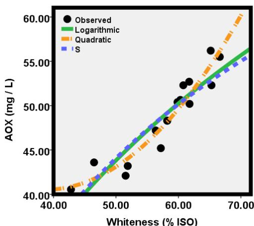
**Fig. 3.** Model equation relationships between pulp whiteness and wastewater AOX content
