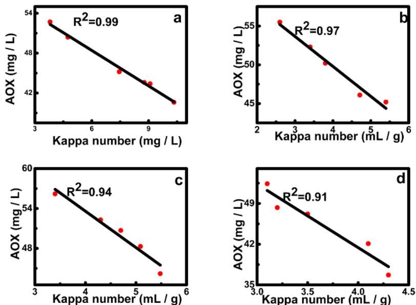
**Fig. 9.** Correlation between pulp Kappa number and wastewater AOX content at different chlorine dioxide delignification stage conditions (a: dosage of chlorine dioxide 0.7 to 3.2%; b: bleaching temperature 40 to 90 °C; c: bleaching time 35 to 85 min; and d: initial pH of chlorine dioxide stage 3 to 11)
