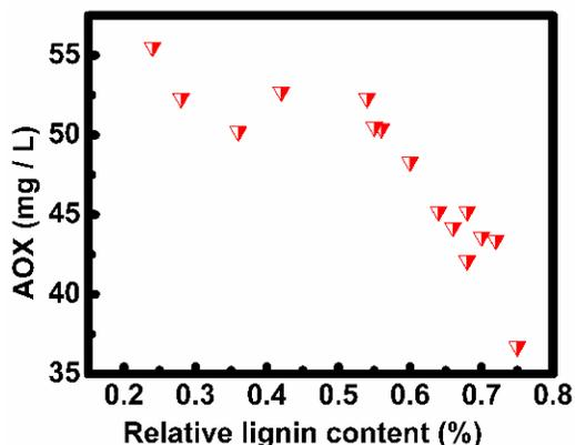
Fig. 2. Correlation between pulp relative lignin content and wastewater AOX content
