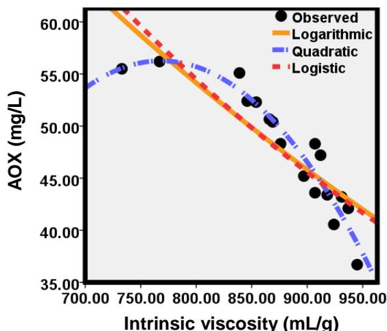
Fig. 7. Model equation correlations between intrinsic pulp viscosity and wastewater AOX content
