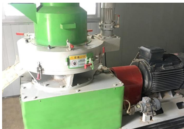
Fig. 1. Biomass pellet mill with horizontal and ring type die
