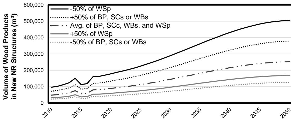
**Fig. 7.** Sensitivity of one numerator (BP, SCs, or WBs) and the denominator (WSp)
