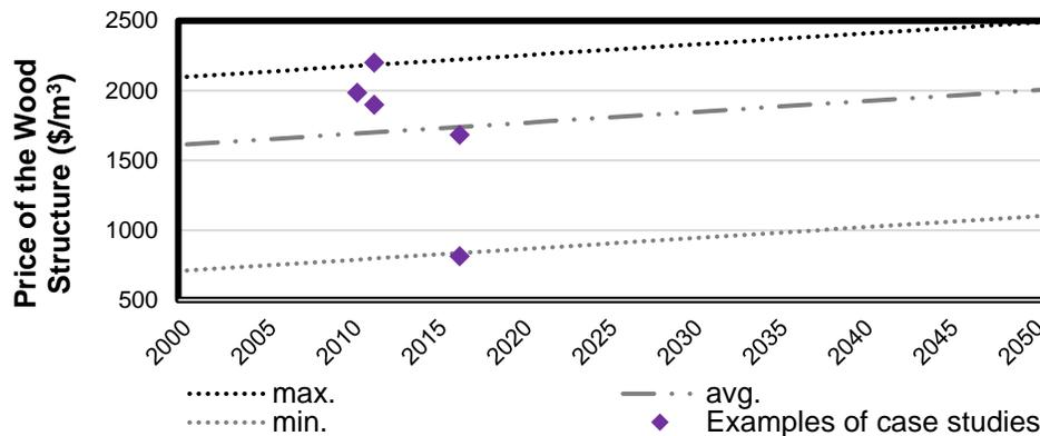
**Fig. 4.** Range of the example of the cost of a wood structure (*WSp*); Linear trend: FEA (2019); case studies: CECOBOIS (2012, 2013), Beaucher (2014, 2017), and Beaucher *et al.* (2018)
