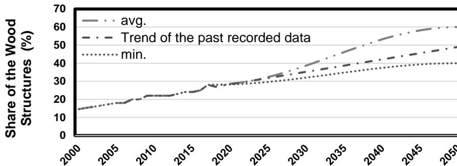
**Fig. S4.** Sensitivity of the share of building with wood structures (WBs) projections (Fig. 5 modified). Historical values: Robichaud (2017); Projections: s-curve scenarios and historical trend
