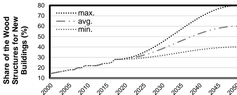
**Fig. 5.** Share of the wood structures for new buildings (*WBs*); Historical values: Robichaud (2017); Projections: s-curve scenarios (Eq. 3)
