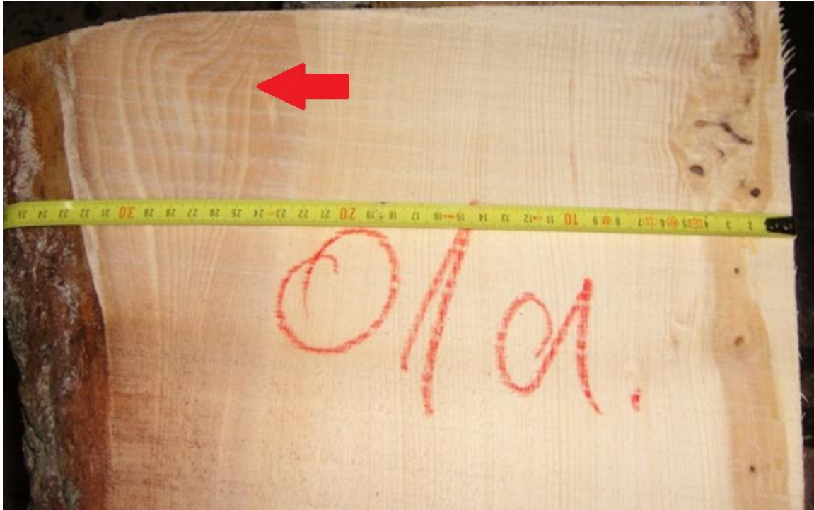
Fig. 5. Timber from resonance tree buttress (arrow indicates fibre deviations)
