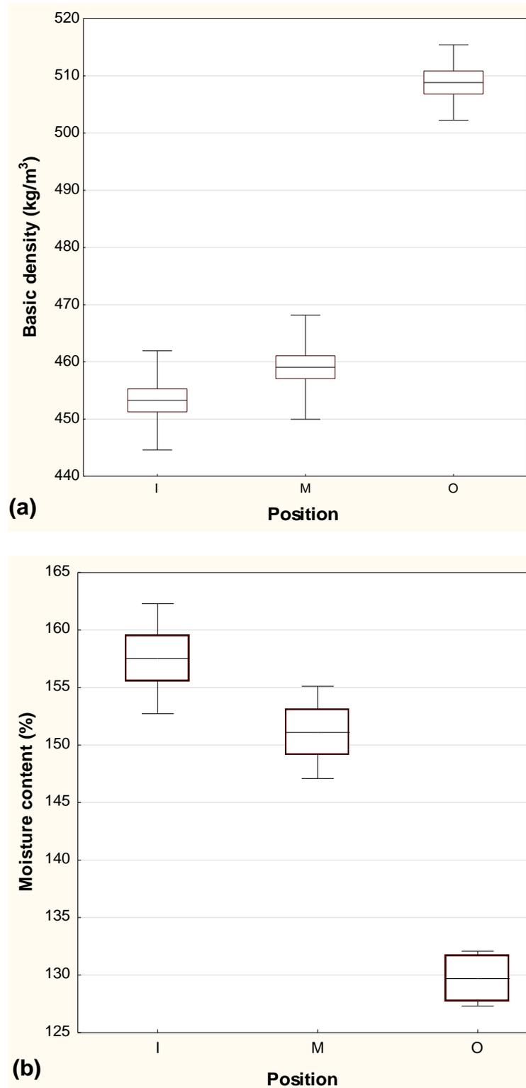
**Fig. 2.** Variation of (a) basic density and (b) moisture content of *E. nitens* as a function of the radial position
