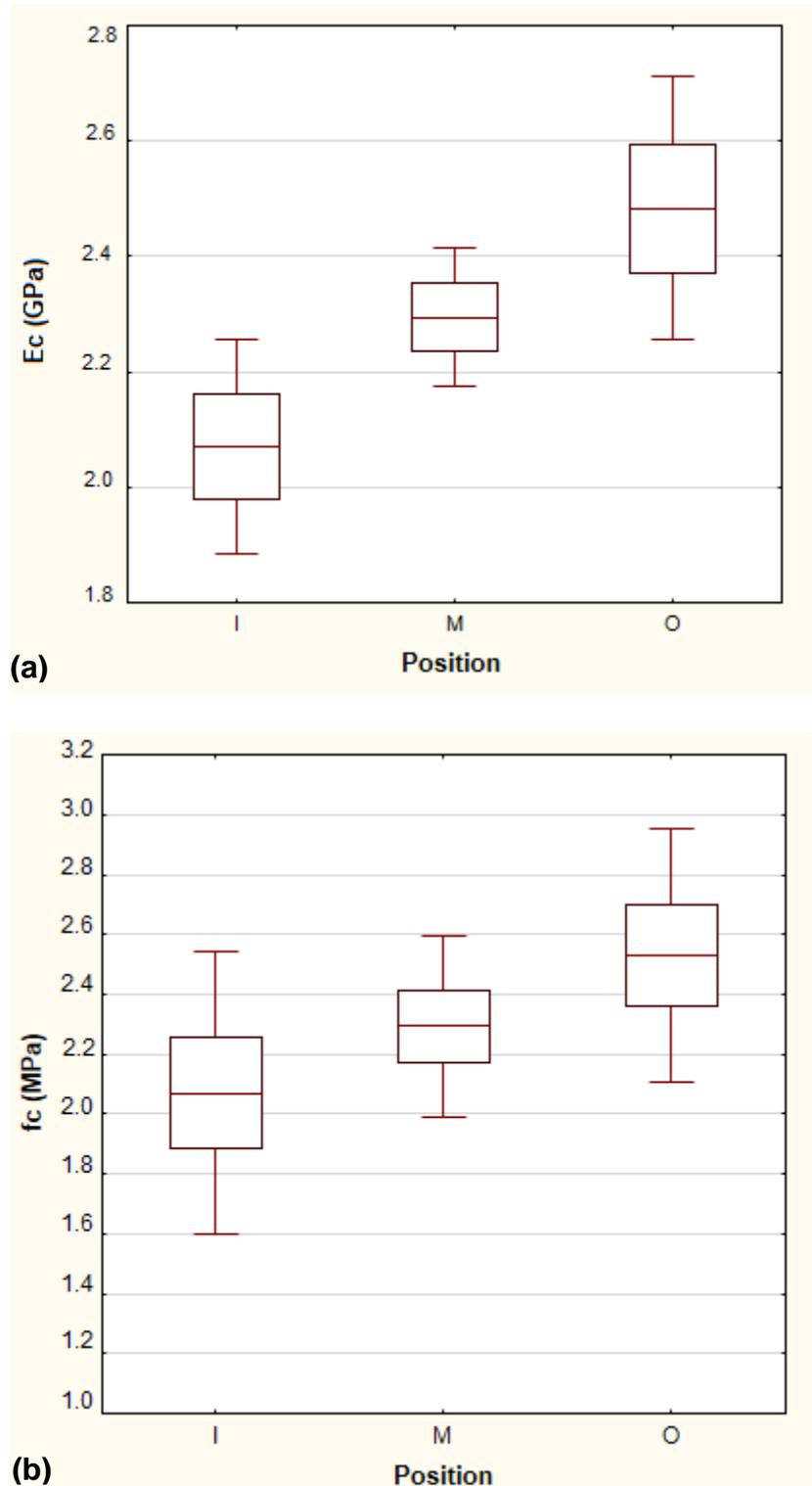
**Fig. 3.** Compressive properties perpendicular to the fiber of *E. nitens* as a function of the radial position: (a) modulus of elasticity and (b) compressive strength
