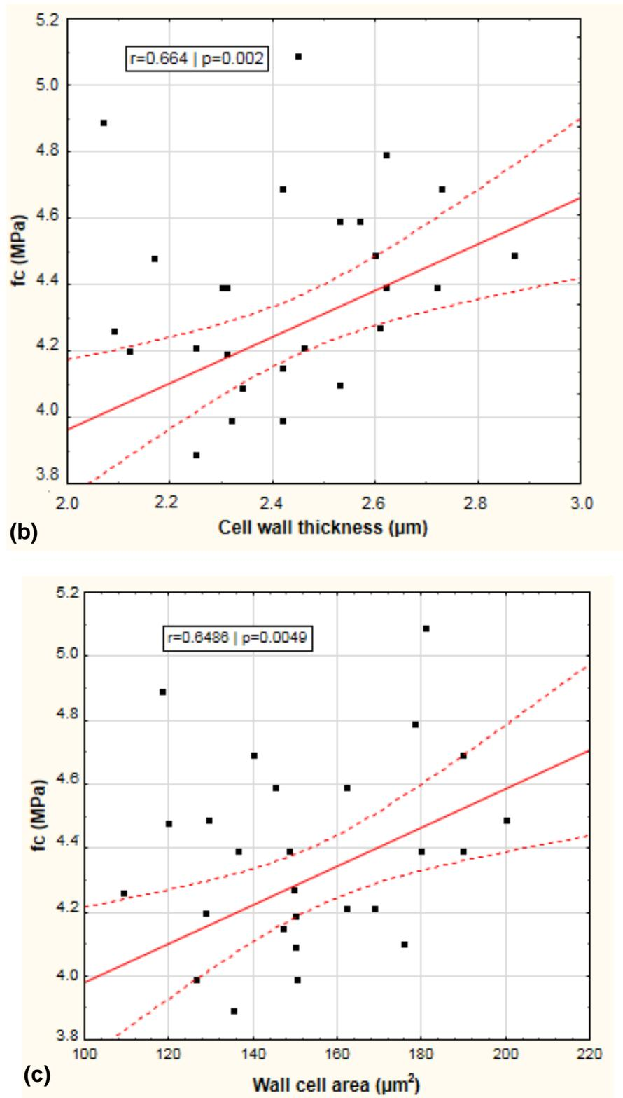
**Fig. 4.** Relationship between compressive strength and (a) basic density, (b) cell wall thickness, and (c) wall cell area
