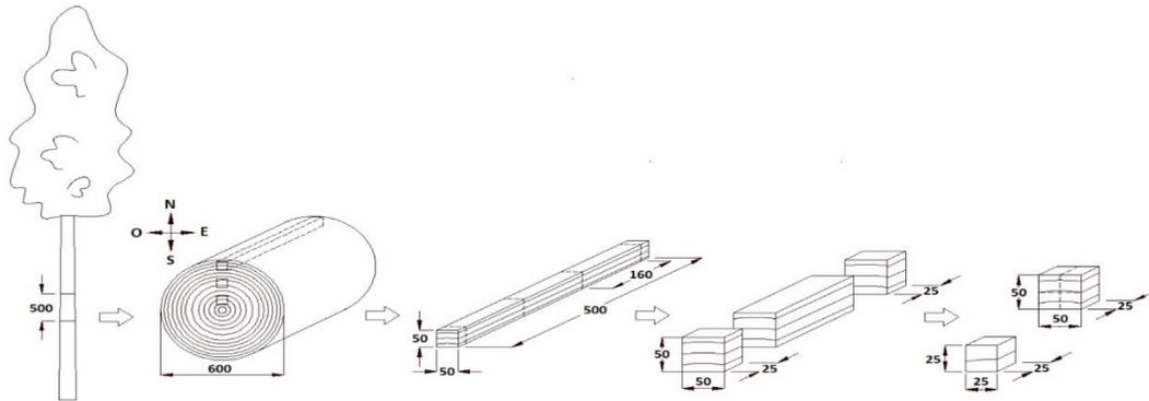
**Fig. 1.** Extraction of the logs at 1.3 m and specimens on the radial distance to the pith of each disk
