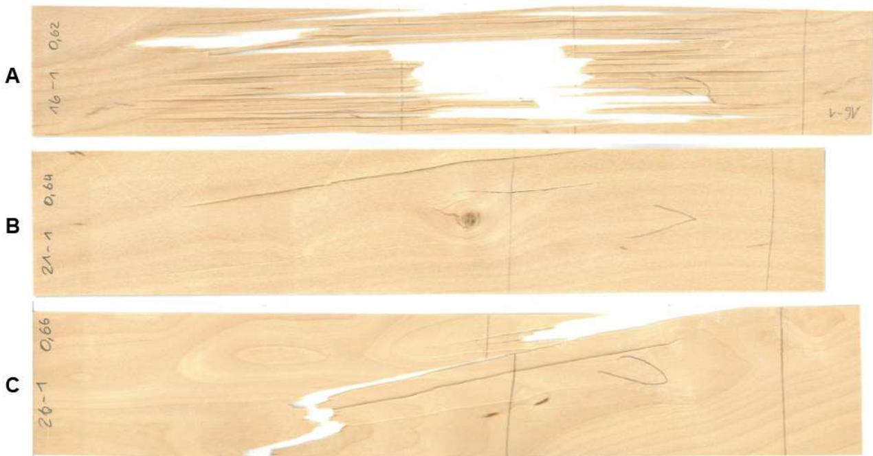
**Fig. 2.** Example veneers for grade A (no defects), B (knots) and C (fiber deviation  $> 15^\circ$ )
