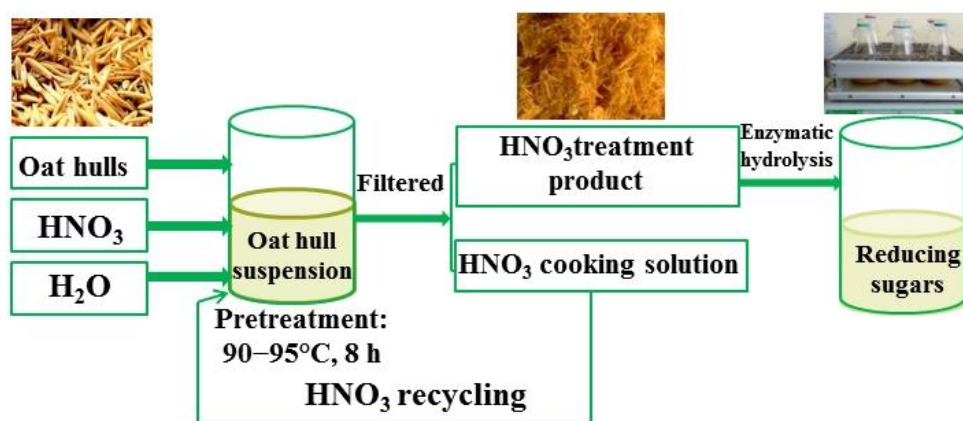
Fig. 2. Illustration of the conversion of oat hulls into reducing sugars through HNO 3 recycling
