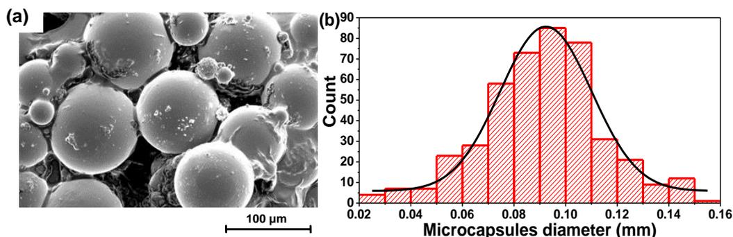
Fig. 2. (a) SEM micrograph of microcapsules; (b) diameter distribution of microcapsules
