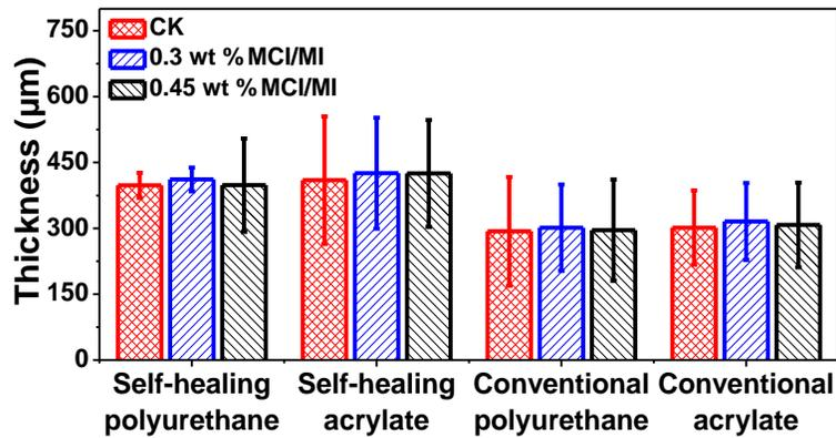
**Fig. 6.** Thickness of coatings; Error bars represent the standard deviation
