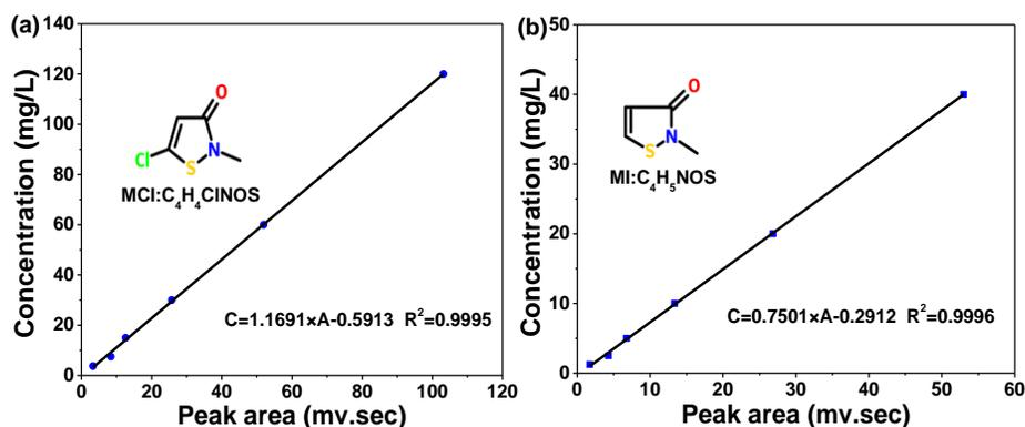
**Fig. 1.** Standard curves of (a) MCI and (b) MI; C is the concentration (mg/L); A is the peak area (mv.sec)
