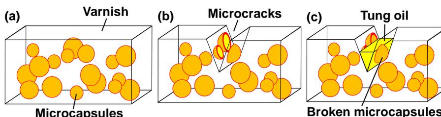
**Fig. 4.** Schematic diagram of self-healing behavior; (a) Not damaged; (b) Damaged; (c) Self-healing
