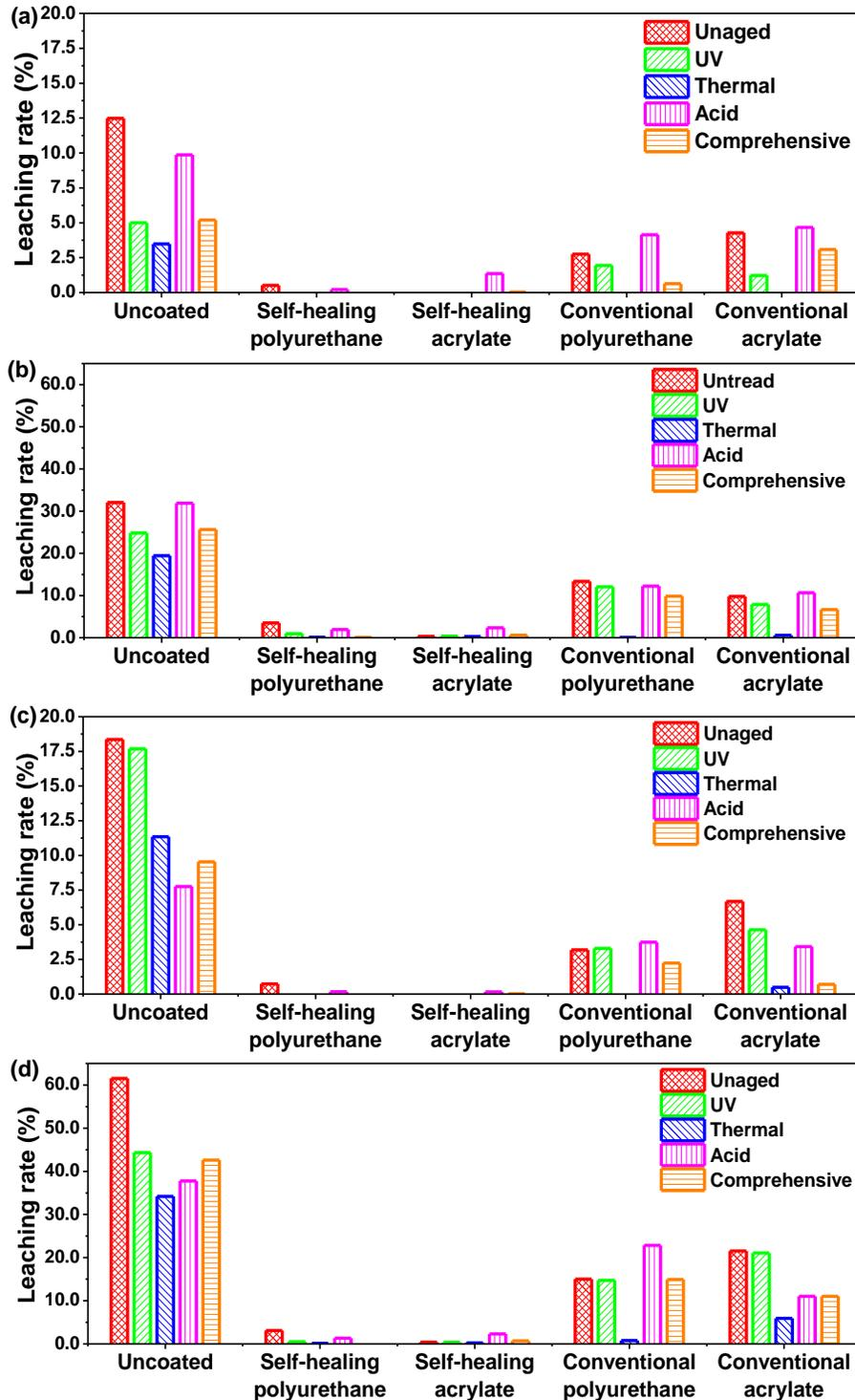
**Fig. 5.** Leaching rates of (a, c) MCI and (b, d) MI from bamboo treated with 0.3 wt% and 0.45 wt% isothiazolinone (MCI/MI) after accelerated aging
