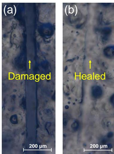
**Fig. 3.** Optical microscope images of damaged self-healing coatings after (a) 0 and (b) 4days
