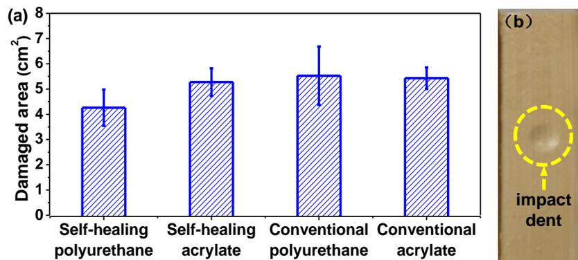
**Fig. 7.** (a) Damaged area of coatings; Error bars represent the standard deviation; (b) Impact dent of coatings
