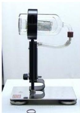
**Fig. 1.** Instrument for rapidly measuring paper ash (reprinted with permissions from German Grenier und Grabner GmbH Co.)
