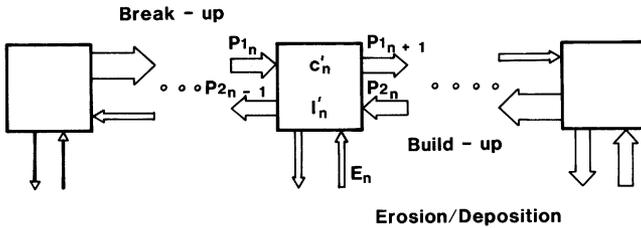
Fig.2: The fibre flocculation concept.
