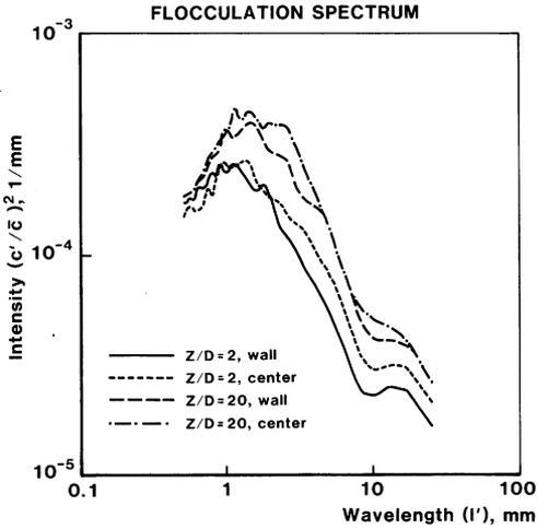
Fig.8: Flocculation spectra, hardwood fibres,  $c=0.17\%$ ,  $u_b=3$  m/s
