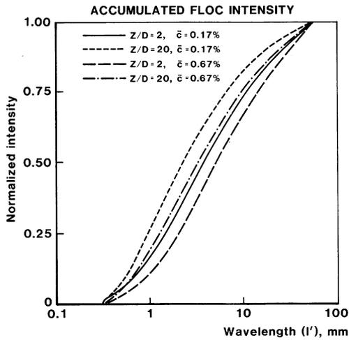
Fig.11: Accumulated floc intensity, softwood fibres,  $u_b=3$  m/s
