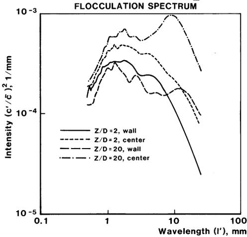
Fig.6: Flocculation spectra, softwood fibres,  $c=0.17\%$ ,  $u_b=1$  m/s
