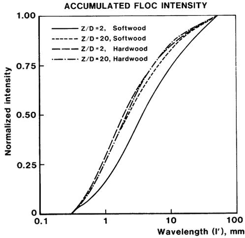
Fig.10: Accumulated floc intensity,  $c=0.17\%$ ,  $u_b=3$  m/s
