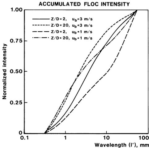
Fig.9: Accumulated floc intensity, softwood fibres,  $c=0.17\%$
