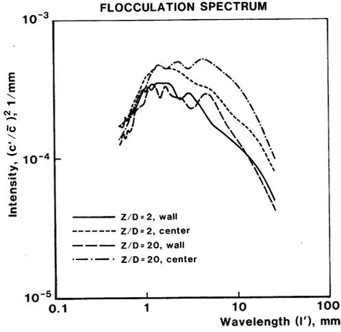
Fig.7: Flocculation spectra, softwood fibres,  $c=0.17\%$ ,  $u_b=3$  m/s
