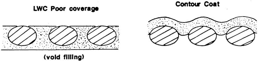
Figure 2. Modification of sheet profile by the application of coating.
