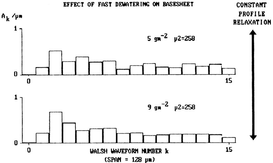
Figure 6(b). Changes in basesheet profile during fast colour dewatering.
