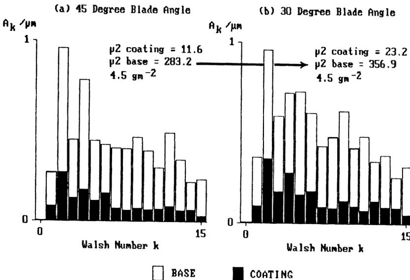
Figure 12. Basesheet roughening due to pressure dewatering.
