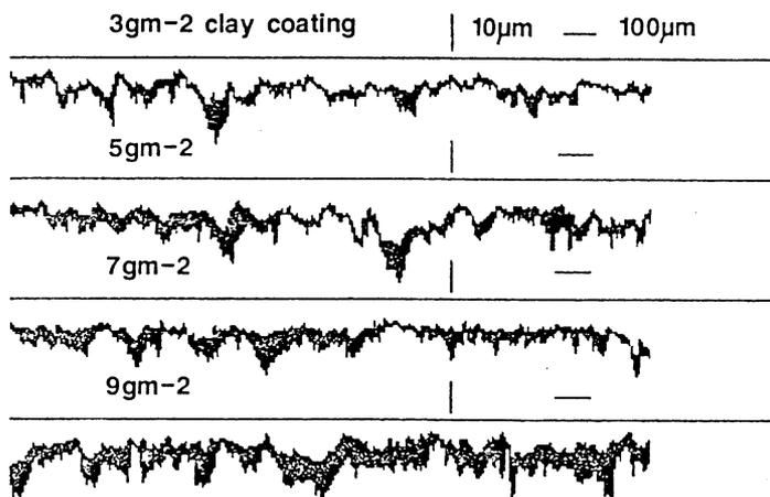
Figure 3. Computer images of the coating layer.
