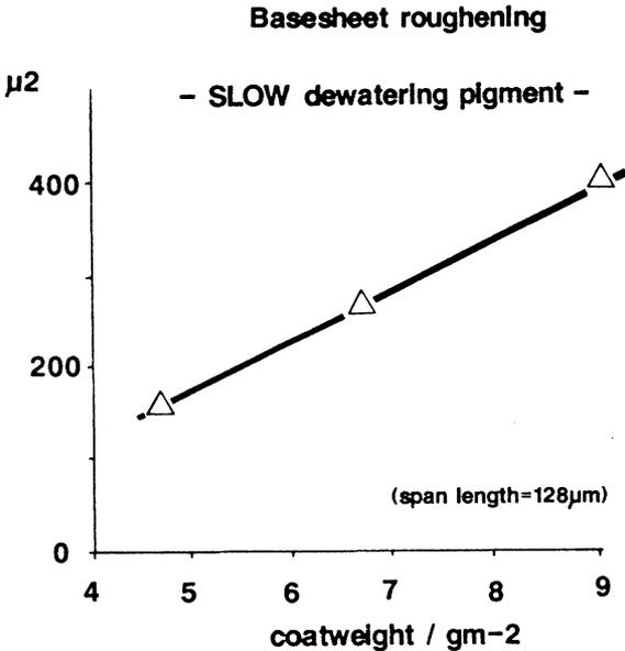
Figure 7(a). Unconstrained basesheet roughening - proportional to LWC coating weight.
