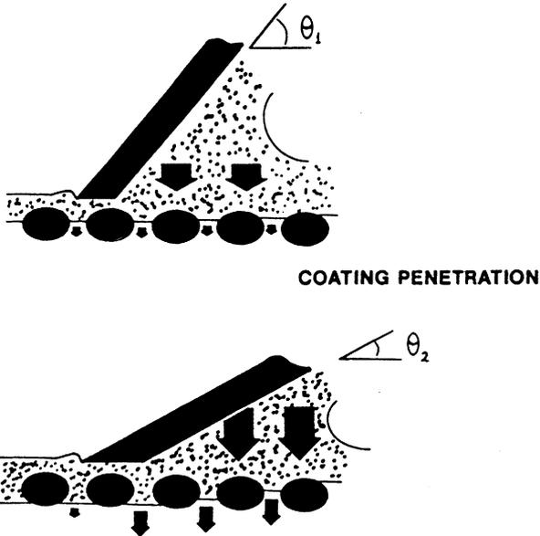
Figure 11. Low angle stiff blade increases pressure dewatering.
