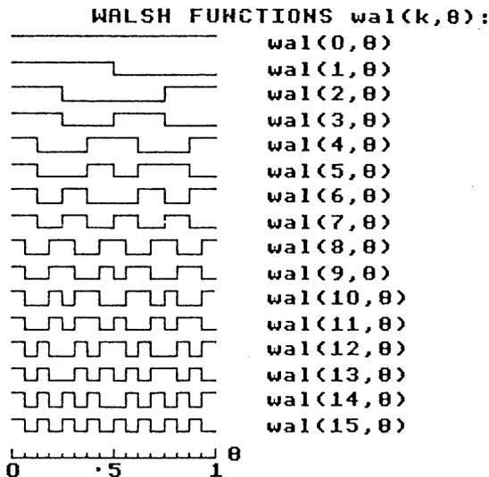
Figure 4. The basis set of 15 Walsh functions used to transform a span length of  $\theta$ .
