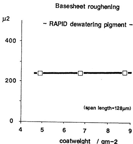
Figure 7(b). Constrained basesheet roughening - independent of coat weight.
