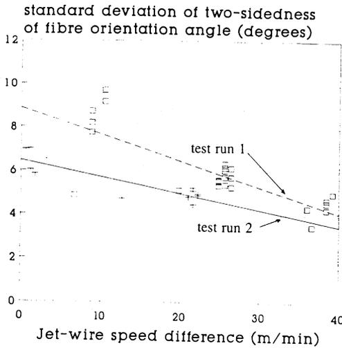
**Fig. 12.** Effect of the jet-wire speed difference on local two-sidedness of the fibre orientation angle. Results from a trial run at KCL.
