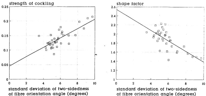
**Fig. 11.** Effect of local two-sidedness of the fibre orientation angle on the strength of cockling and the shape of the cockles. Results from a trial run at KCL.
