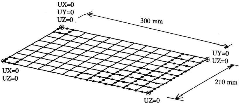
**Fig. 5.** The element model used. The properties of each element are random.
