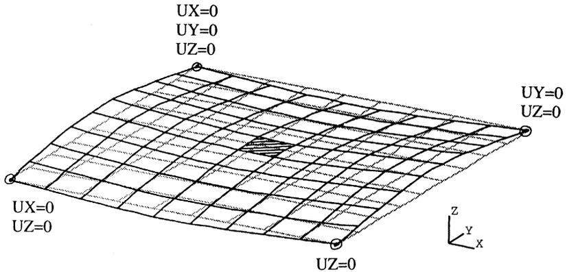
**Fig. 3.** Buckling of an isotropic square plate to form a saddle surface, when only the middle element has non-zero hygroexpansivity.
