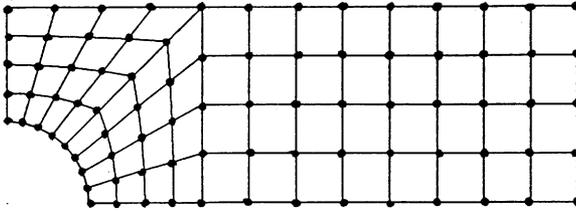
**Fig. 1.** Division of a continuous structure into elements.
