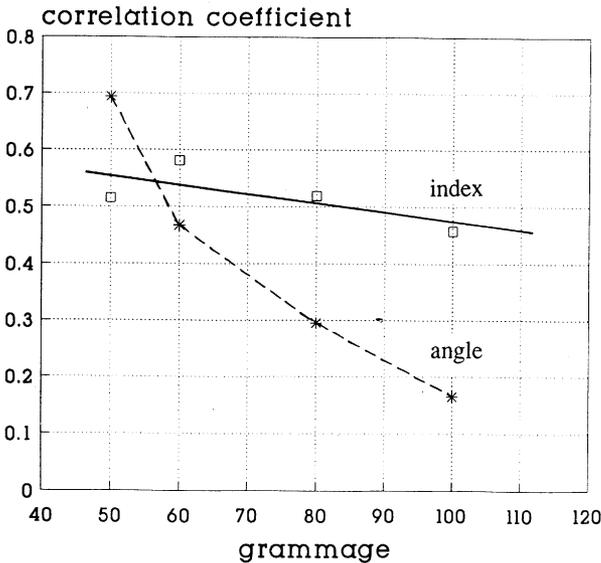
**Fig. 9.** Correlation of orientation between the different sides of paper as a function of grammage. All papers were fabricated on fourdrinier paper machines, either at KCL or at a paper mill.
