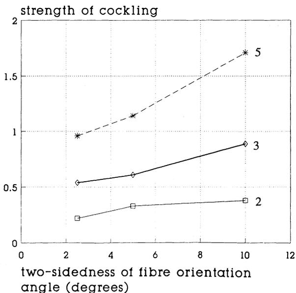
**Fig. 6.** Strength of cockling as a function of local two-sidedness of the fibre orientation angle. The average orientation ratio is 2, 3 or 5.
