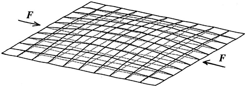
**Fig. 2.** Buckling of a uniaxially compressed clamped square plate.
