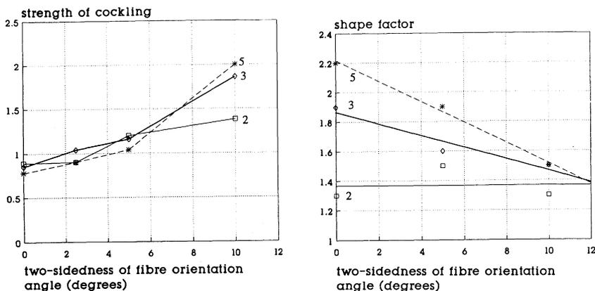
**Fig. 8.** Effect of local two-sidedness of the fibre orientation angle and orientation ratio on the strength and shape of cockles. The average orientation ratio is 2, 3 or 5 and the two-sidedness 10%.
