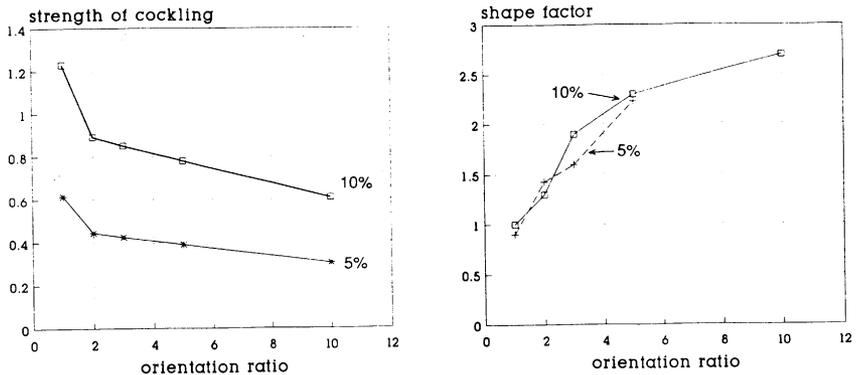
**Fig. 7.** Strength of cockling and the shape factor as a function of orientation ratio.
