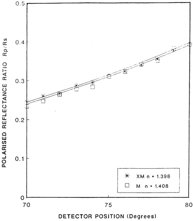
FIGURE 8 The polarised reflectance ratio  $R_p/R_s$  values as a function of detector position for the data illustrated in Figure 7. Symbols indicate experimental data points; full lines are calculated.
