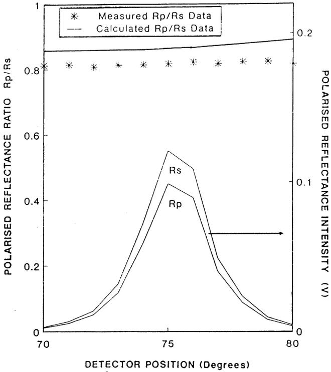
FIGURE 10 Similar data to that given in Figure 9 but for gold vapour deposited on a coated paper surface.
