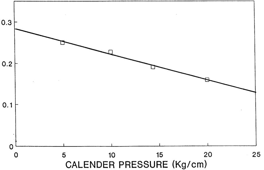
Figure 1: Effect of calender pressure on fractional void in surface layer.
