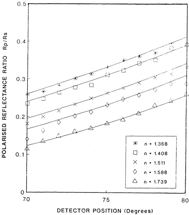
FIGURE 6 A comparison of measured and calculated values for the polarised reflectance ratio ( $R_p/R_s$ ) for coated surfaces with a range of refractive index values. Data points are indicated by symbols; full lines are calculated values.
