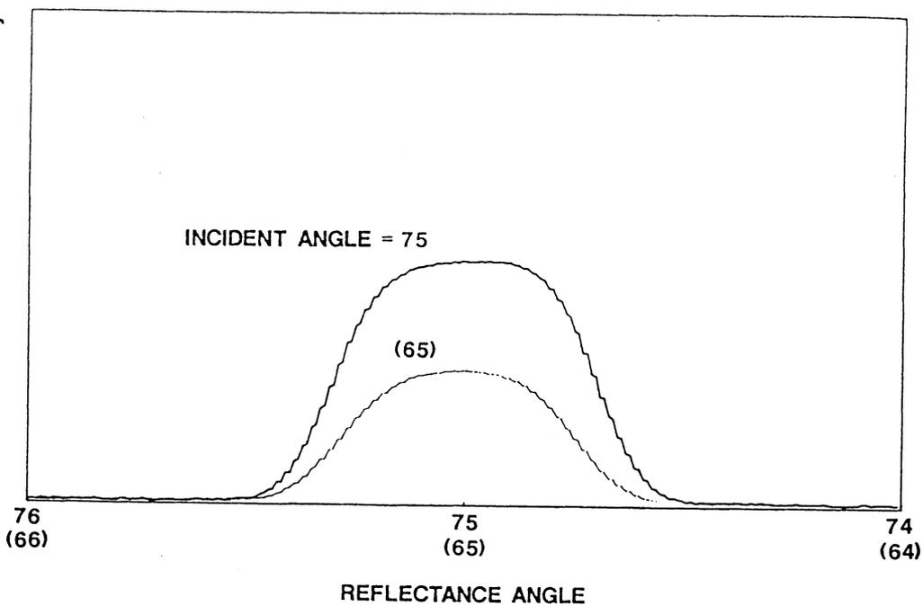
FIGURE 2 Response of reflection goniophotometer using polished black glass: (incident angle  $65^\circ$  and  $75^\circ$ ).
