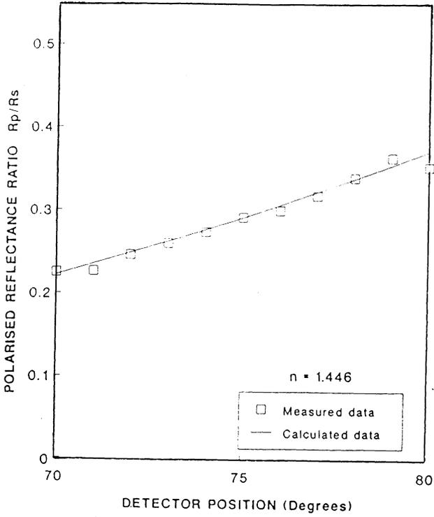
FIGURE 4 The polarised reflectance ratio  $R_p/R_s$  as a function of detector position for the coated paper sample illustrated in Figure 3.
