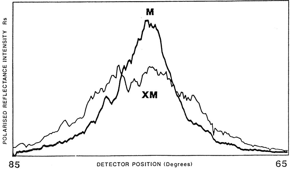
FIGURE 7 The reflected intensity distribution from coated paper relative to the direction of sheet formation. M = machine direction; XM = cross-machine direction.
