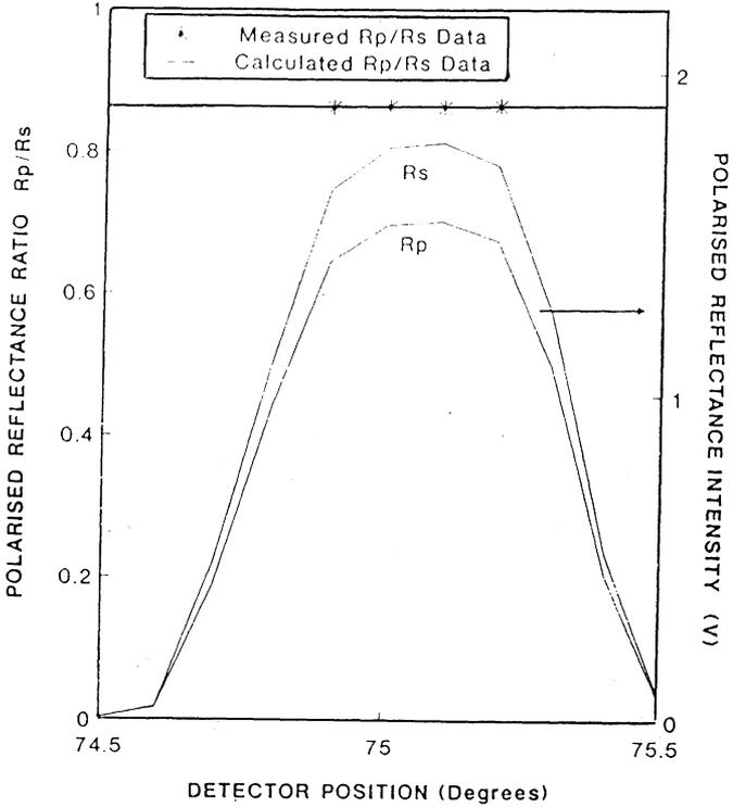
FIGURE 9 Polarised reflectance from a vapour deposited film of gold on a smooth plastic substrate. The R.H. axis refers to the measured intensities given in detector output voltages. The L.H. axis refers to the ratios  $R_p/R_s$  both measured from the curves and calculated from  $n=0.256$   $k=2.126$ .
