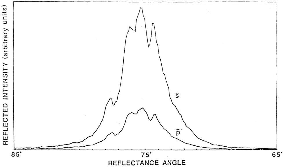
FIGURE 3 The reflected intensity from coated paper as a function of detector angle. The incident light is polarised in either the s or p mode.
