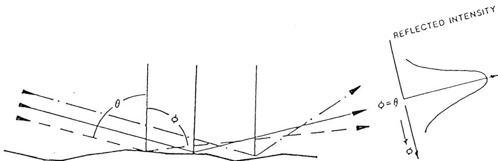
Schematic cross section through a coated surface with reflecting facets
