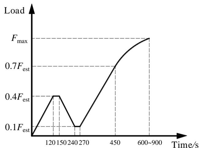
Fig. 3. Loading procedure according to EN 26891 (1991)
