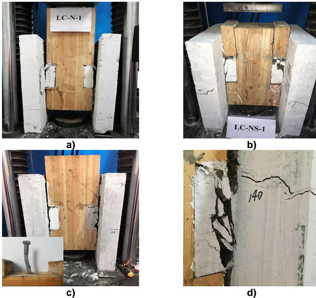
**Fig. 4.** Failure phenomena of the notched connectors: a) shear fracture of the concrete; b) shear fracture of the timber; c) shear fracture of the concrete with screw from bending; and d) diagonal-compression failure of the concrete.
