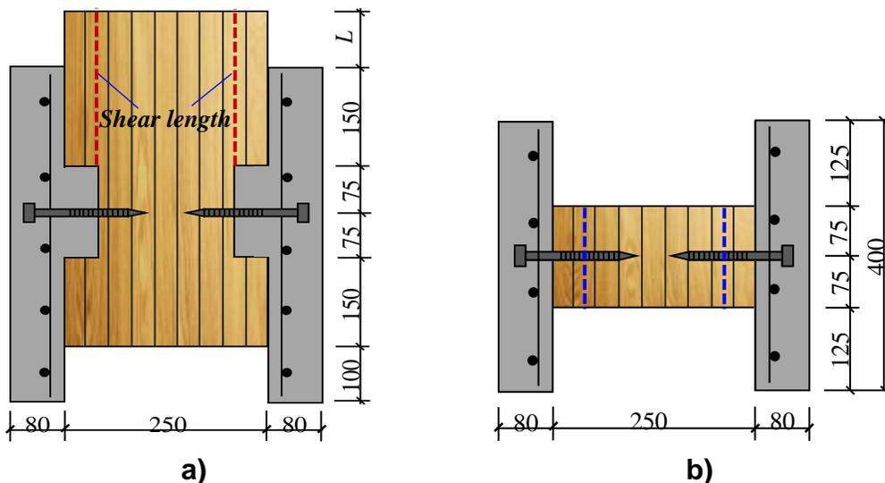
**Fig. 1.** Dimensions of push-out specimens (unit: mm): a) front view of specimens; b) top view of specimens. Note: In test series NC-N-1, LC-N-1, and LC-NS-4,  $L$  was 200 mm; in specimens LC-NS-1 through LC-NS-3,  $L$  was 0 mm, 50 mm, and 125 mm, respectively.
