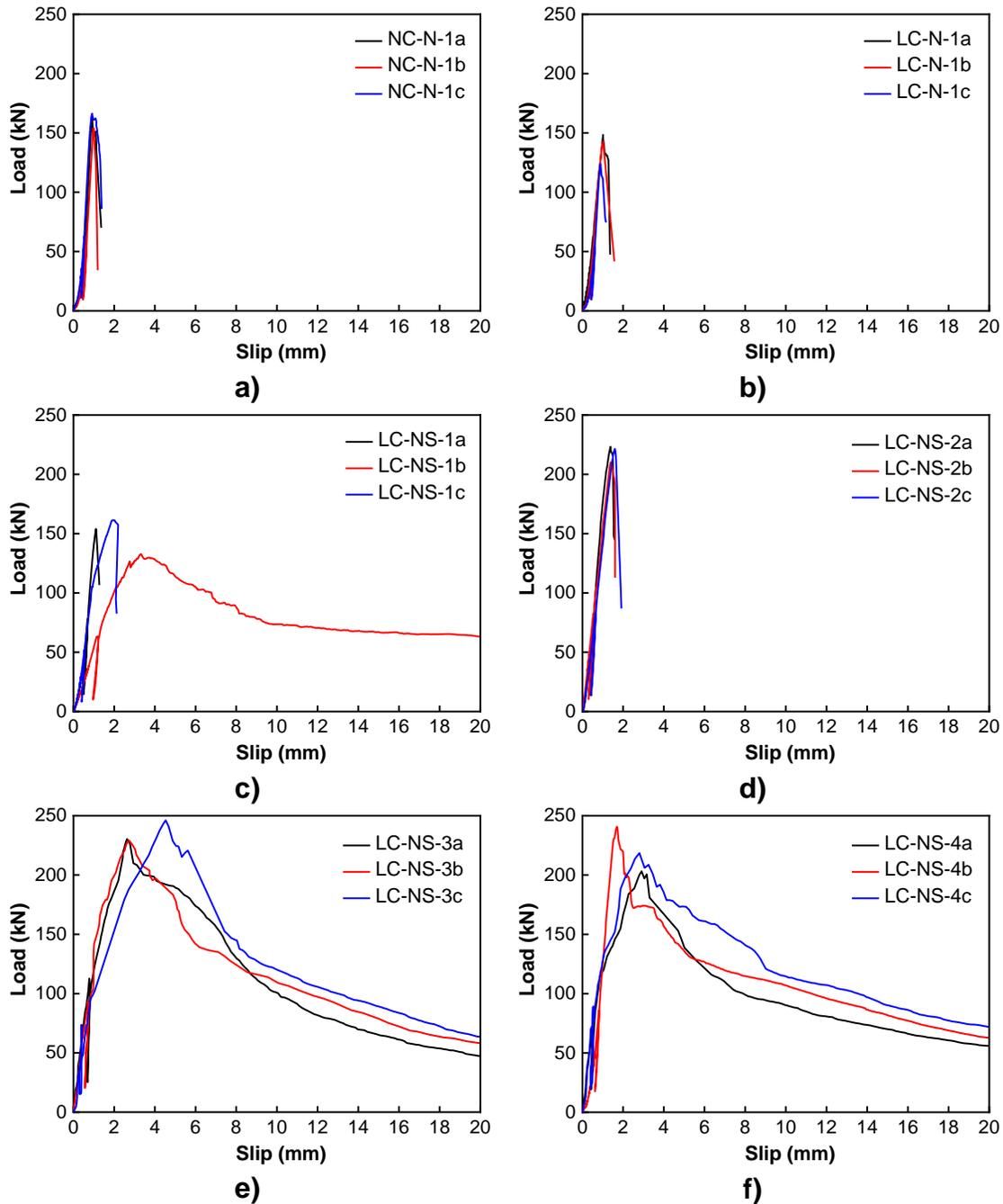
**Fig. 5.** Load-slip curves for the notched connectors: a) Test series NC-N-1; b) Test series LC-N-1; c) Test series LC-NS-1; d) Test series LC-NS-2; e) Test series LC-NS-3; and f) Test series LC-NS-4
