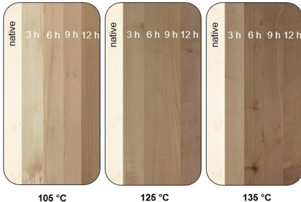
Fig. 4. Changes in the colour of maple wood during thermal modification
