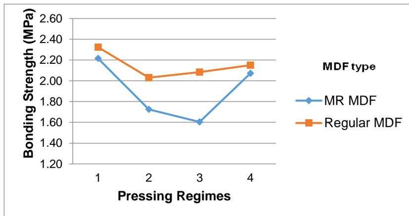
**Fig. 9.** Influence of substrate type and pressing regime on the bonding strength of oak veneer
