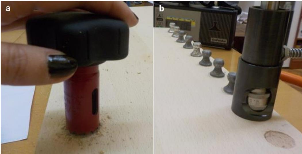
**Fig. 4.** Cutting veneer before the pull-out of dollies (a) and removal of dollies (b)
