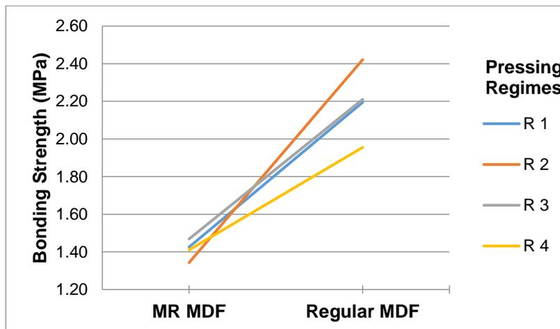
Fig. 5. Influence of substrate type and pressing regime on the bonding strength of beech veneer
