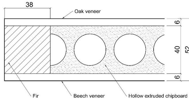
**Fig. 3.** Cross-section of door construction (dimensions in mm)
