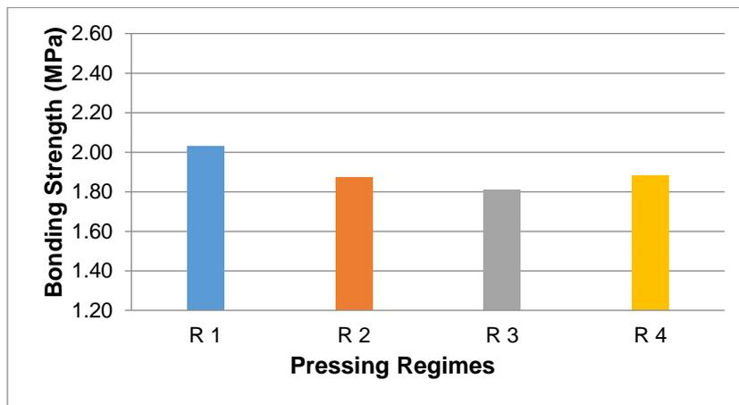
**Fig. 7.** Influence of pressing regime on the bonding strength regardless of substrate type or veneer species
