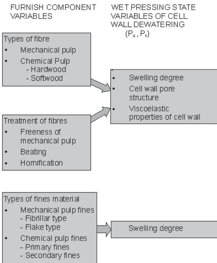
**Figure 13** A schematic illustration of furnish and wet pressing state variables.
