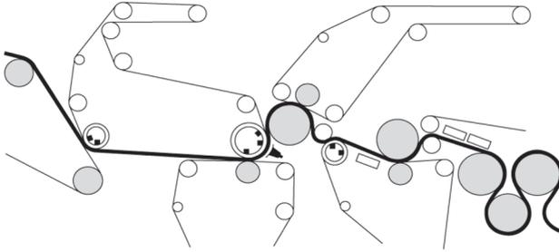
**Figure 2** A four-nip press section of a printing paper machine.
