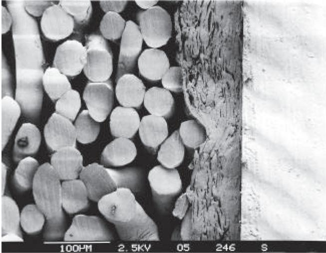
**Figure 6** SEM micrograph of felt/paper interface, magnified 230× [56].
