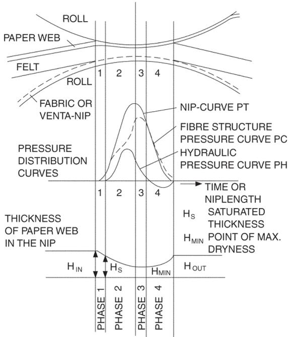
**Figure 3** The four phases of the nip process according to Nilsson and Larsson [7].
