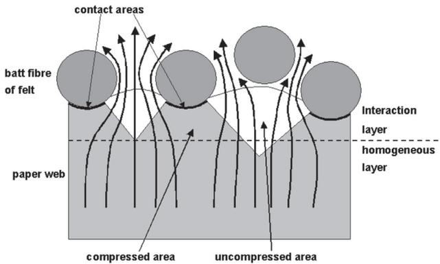
**Figure 4** Hypothesis on the interaction between the felt and the web and its influence on the water flow inside the web [21].
