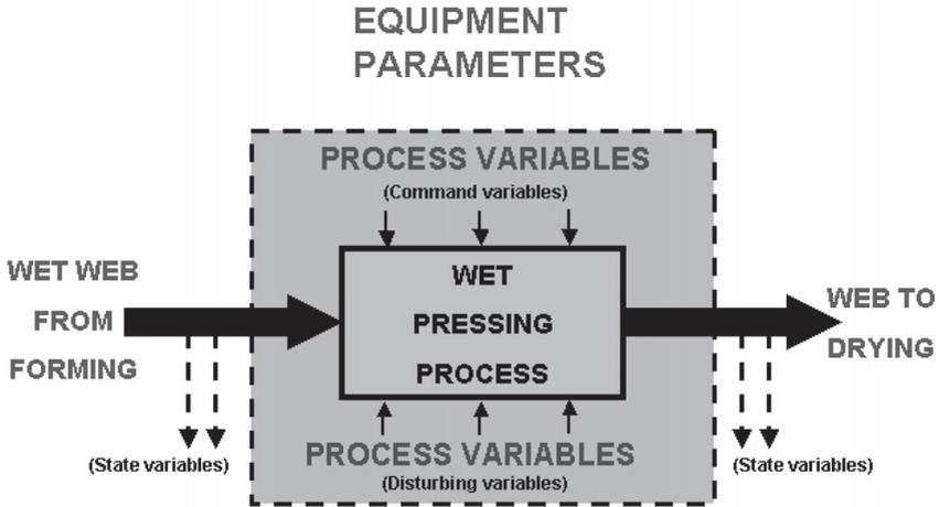
**Figure 1** Conceptual process scheme of wet pressing.
