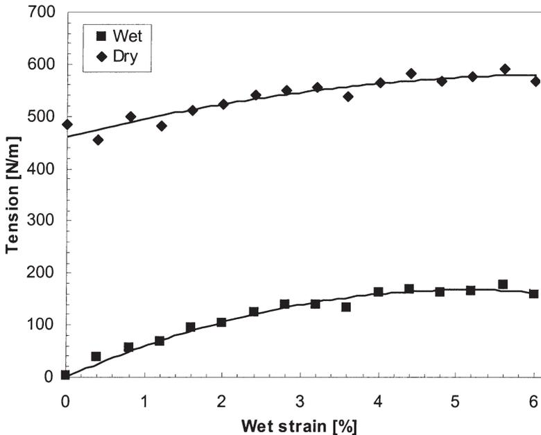
**Figure 3** Tension of wet and dry paper vs. the level of wet strain.
