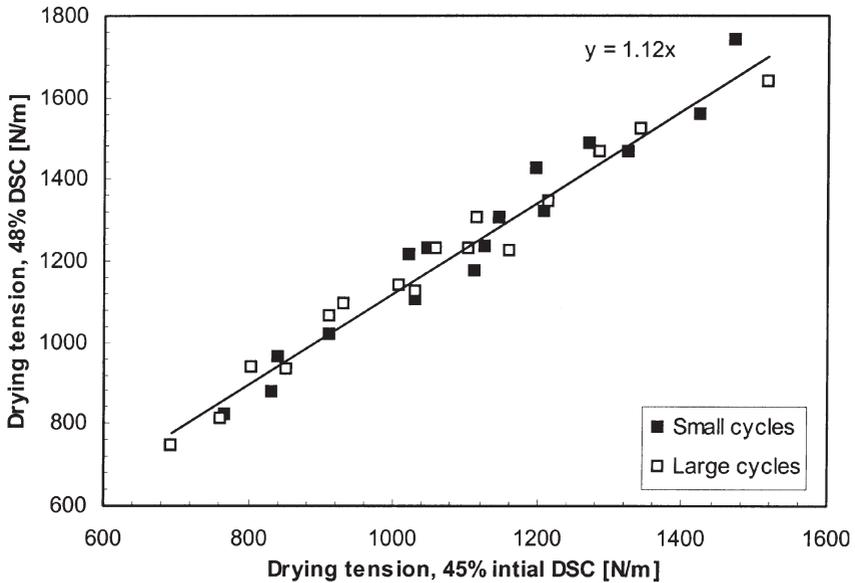
**Figure 10** Drying tension of samples with 48% initial dry solids content vs. drying tension of the 45% samples.
