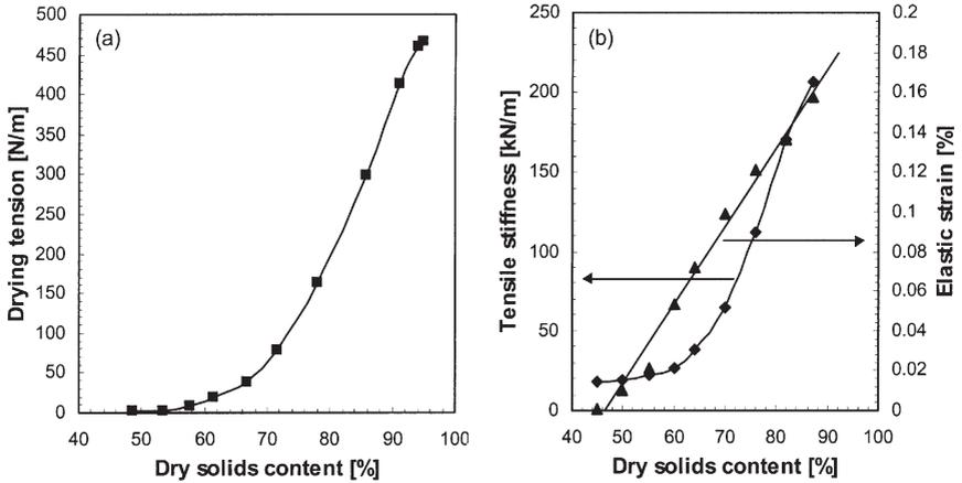
**Figure 1** Drying tension (a), tensile stiffness and elastic strain (b) vs. dry solids content in uniaxial restraint drying.
