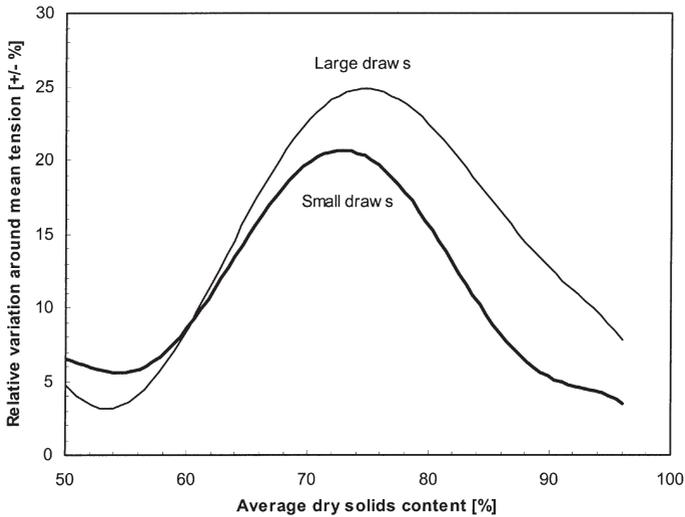
**Figure 9** Relative tension variation around the mean tension vs. average dry solids content of paper. Large draws mean maximum level of the all draws 1–4 in Figure 8, and respectively small draws mean minimum level of the draws.
