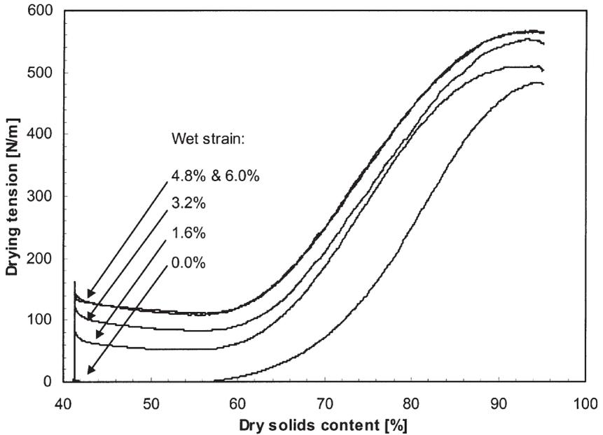
**Figure 2** Drying tension vs. dry solids content for different wet strain levels.
