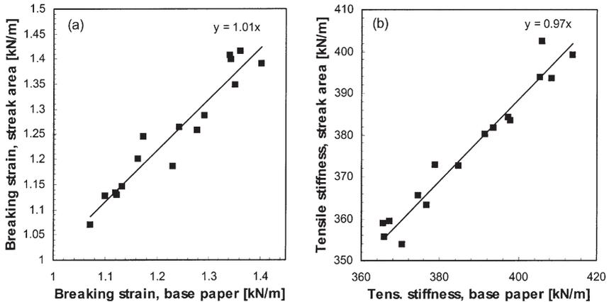
**Figure 15** Breaking strain (a) and tensile stiffness (b) of the area of moisture streak vs. breaking strain and tensile stiffness of base paper in pilot drying machine.
