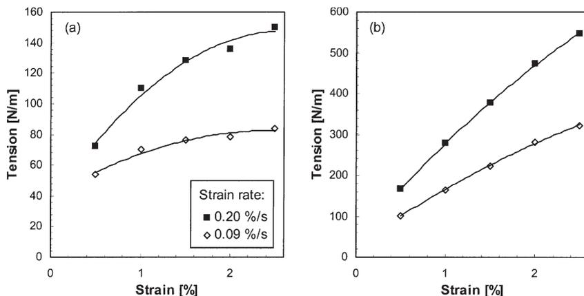
**Figure 5** Maximum tension and relaxed tension vs. initial strain. Specimens are restraint dried to 48% (a) and 72% (b) dry solids content before 0.17%/s straining. Relaxation results correspond 0.09%/s strain rate.
