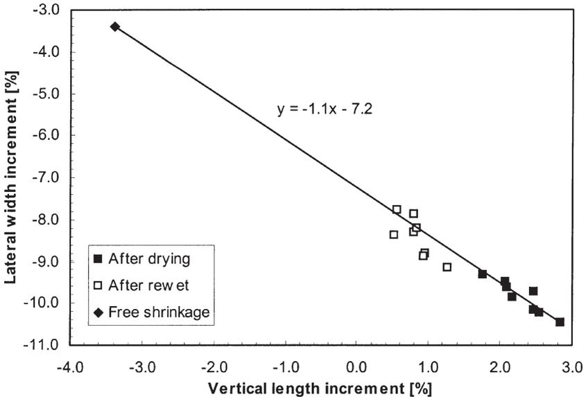
Figure 14 Vertical length and lateral width of samples after drying and after rewet.
