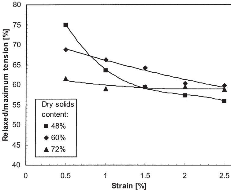
**Figure 6** Ratio of relaxed tension to maximum tension vs. initial strain for different dry solids contents.
