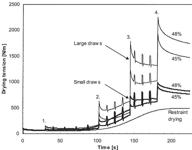
**Figure 8** Drying tension vs. drying time. 1.5% wet strain is applied at 45% and 48% dry solids contents. Draws 1–4 are applied at dry solids contents 51% and 54% (0.1% or 0.5% strain), 66% and 70% (0.1% or 0.5% strain), 80% and 85% (0.1% or 0.5% strain), 91% and 94% (0.1% or 0.3% strain). The amplitude of small load-unload cycles is either 0.05% (shown in figure) or 0.1%.
