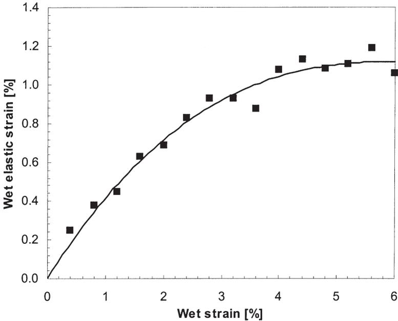
Figure 4 Wet elastic strain vs. wet strain at 41% dry solids content.
