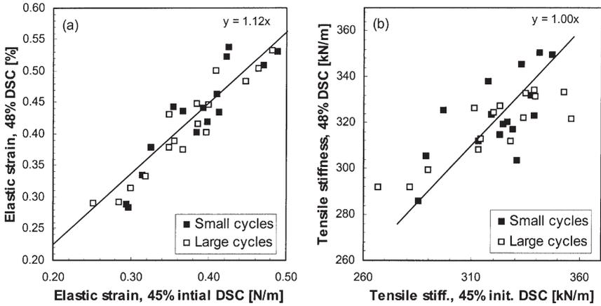
**Figure 12** Elastic strain (a) and tensile stiffness (b) of the 45% and 48% sample sets after drying.
