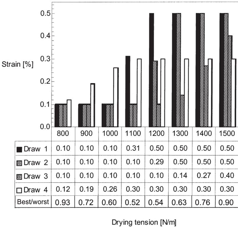
**Figure 11** Optimal draws for fixed drying tensions to minimize tension variation in dry paper between areas of different initial dry solids contents (45% and 48%). The draws number 1, 2 and 3 are limited between 0.1–0.5% and the draw number 4 between 0.1–0.3%. Best/worst-ratio shows relative difference between tension and the variations of best and worst (not shown) setups.
