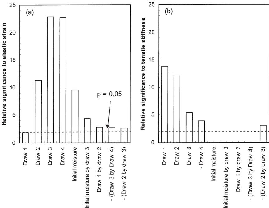
**Figure 13** Statistical significance of factorial analysis parameters to elastic strain (a) and tensile stiffness (b) of the dry paper. Dashed line shows 95% level of confidence.
