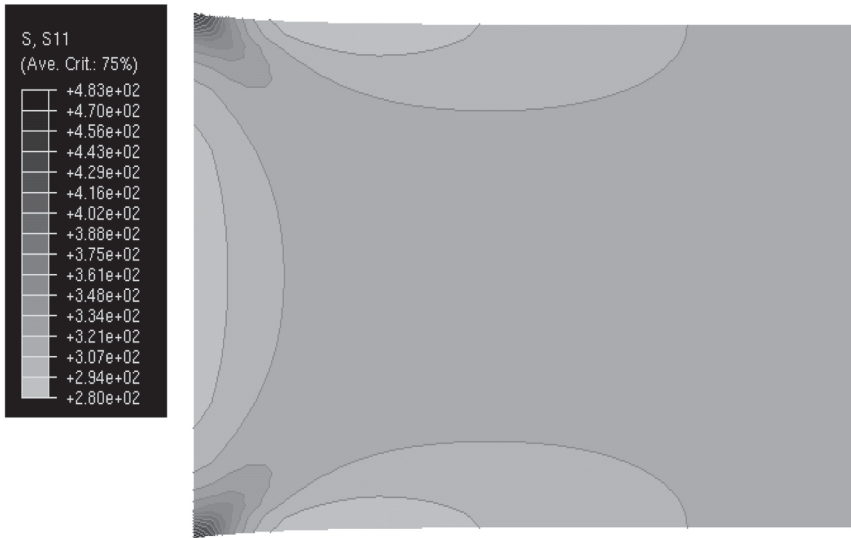
Figure 10 Modelled machine directional stresses induced in the web in an open draw. A monochrome spectrum symbolizes different tension levels. The darker areas are more tense than lighter areas. The left side of the simulated web is fixed and the web is stretched to the right.
