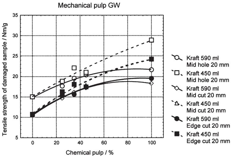
**Figure 6** The effect of defect shape and size on paper strength at various chemical pulp (bleached soft wood/pine kraft) addition levels. Mechanical pulp is GW. Specimen width 50 mm.
