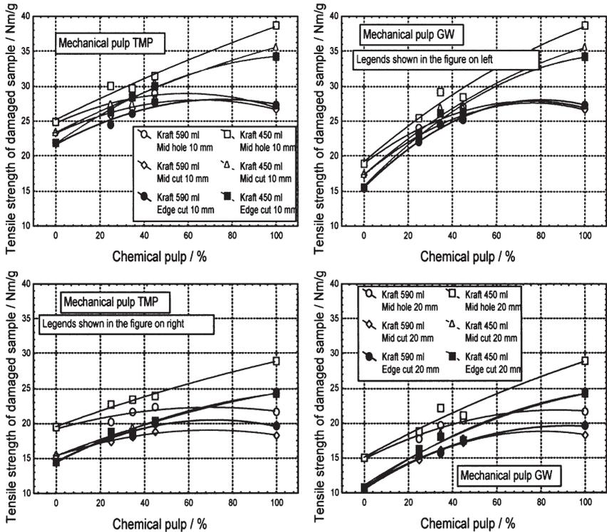
**Figure 7** The effect of defect shape and defect size on paper strength at various chemical (bleached soft wood/pine kraft) pulp addition levels. TMP (left) and GW based sheets compared.
