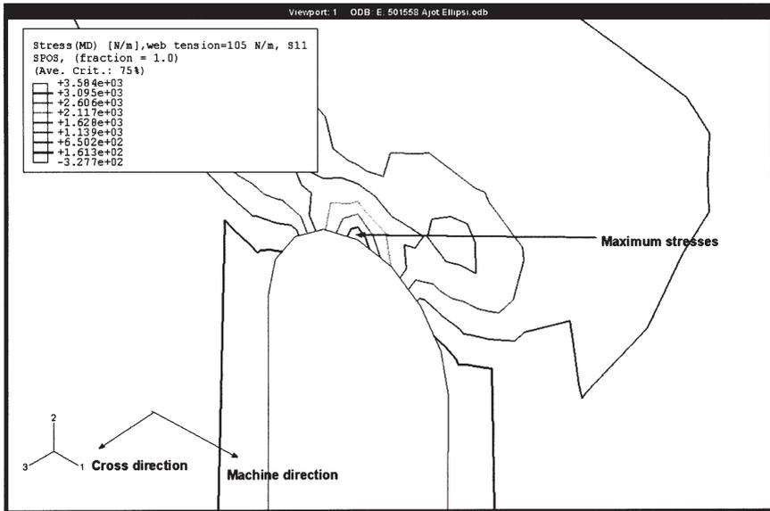
Figure 16 The dependency between web tension and maximum stress around a cut.
