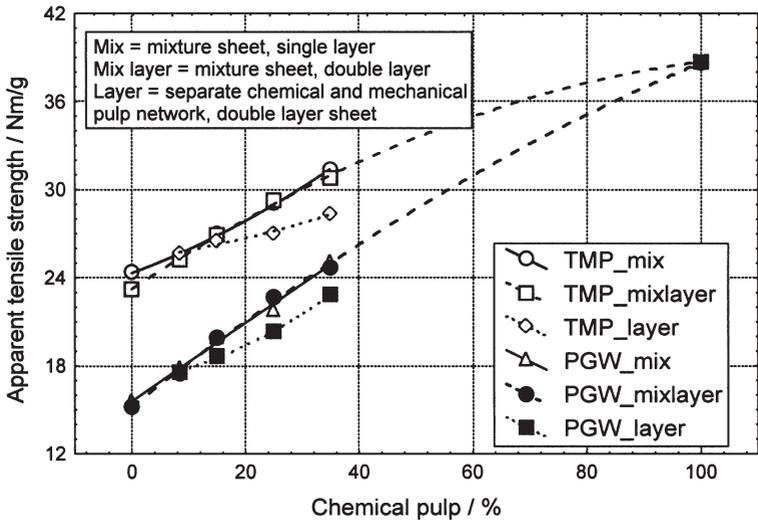
Figure 11 Apparent tensile strength of single and double layered laboratory sheets. Chemical pulp was beaten in laboratory (Valley) to CSF 630 ml.
