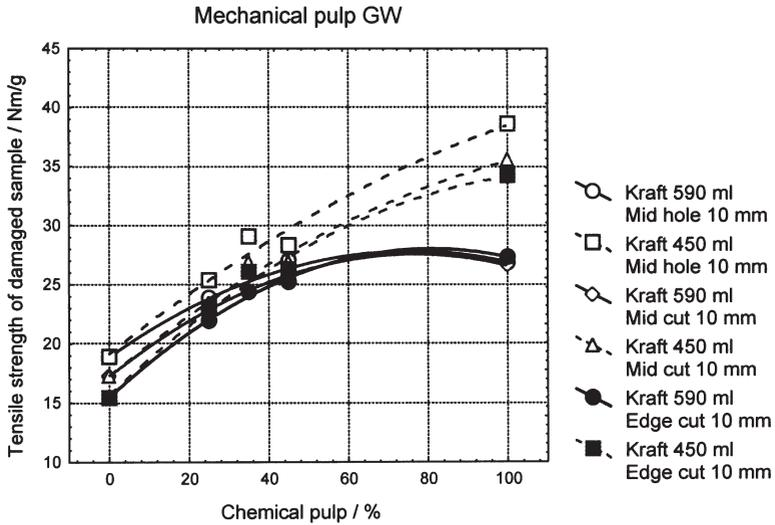
**Figure 5** The effect of defect shape and size on paper strength at various chemical pulp (bleached soft wood/pine kraft) addition levels. Mechanical pulp is GW. Specimen width 50 mm.
