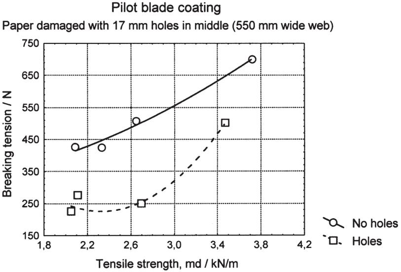
**Figure 1** An example of the effect of defects on breaking tension on a pilot coating machine with different types of base papers.
