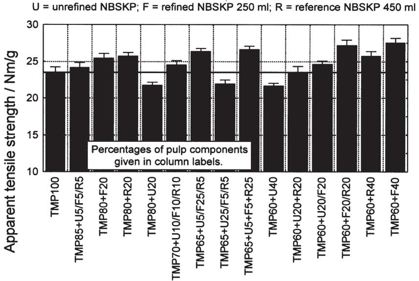
**Figure 8** The effect of chemical pulp beating and content on tensile strength of damaged TMP based paper. Values in column labels after each abbreviation of pulp name give the percentage shares of respective components.
