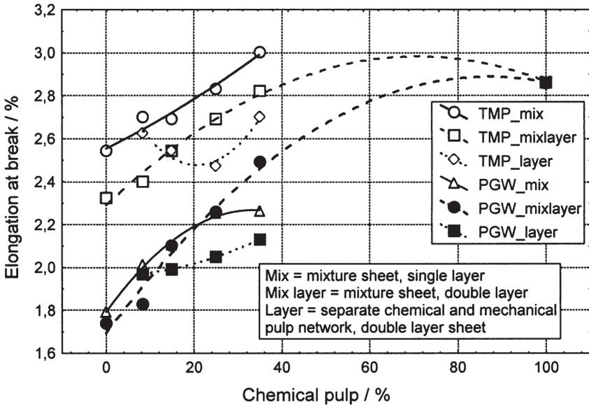
Figure 12 Elongation at break of single and double layered laboratory sheets. Chemical pulp was beaten in laboratory (Valley) to CSF 630 ml.
