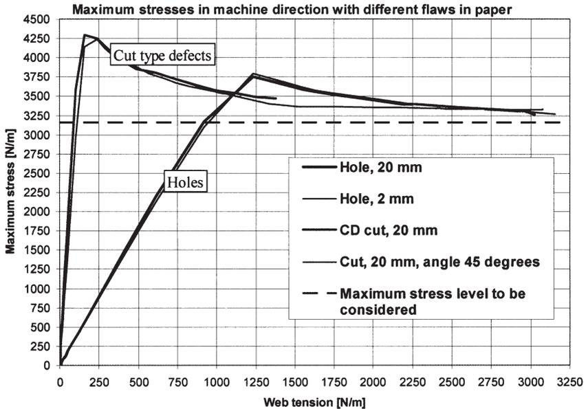
**Figure 13** The dependency between web tension and maximum stress around defect.
