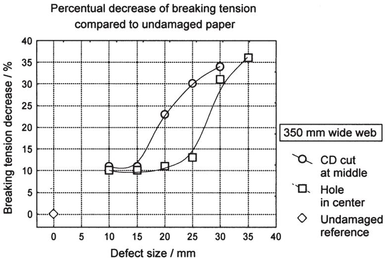
**Figure 2** An example of the effect of defect shape and size on tension at brake in blade coating.
