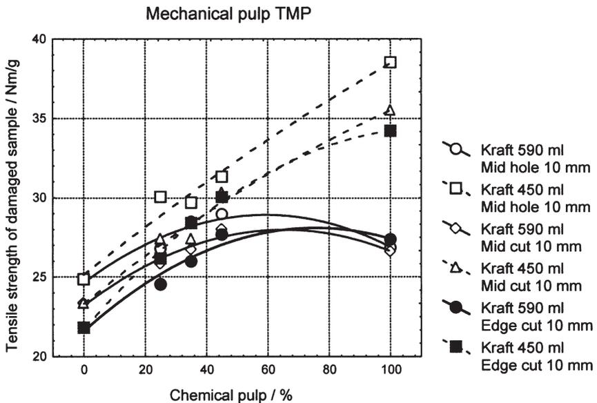
**Figure 3** The effect of defect shape and size on paper strength at various chemical pulp (bleached soft wood/pine kraft) addition levels. Mechanical pulp is TMP. Specimen width 50 mm.
