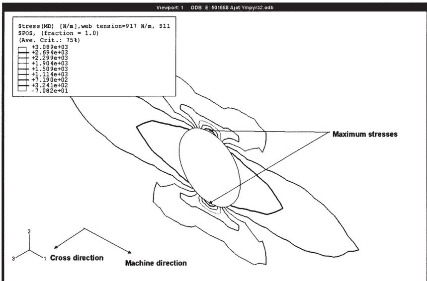
Figure 15 The dependency between web tension and maximum stress around a hole.
