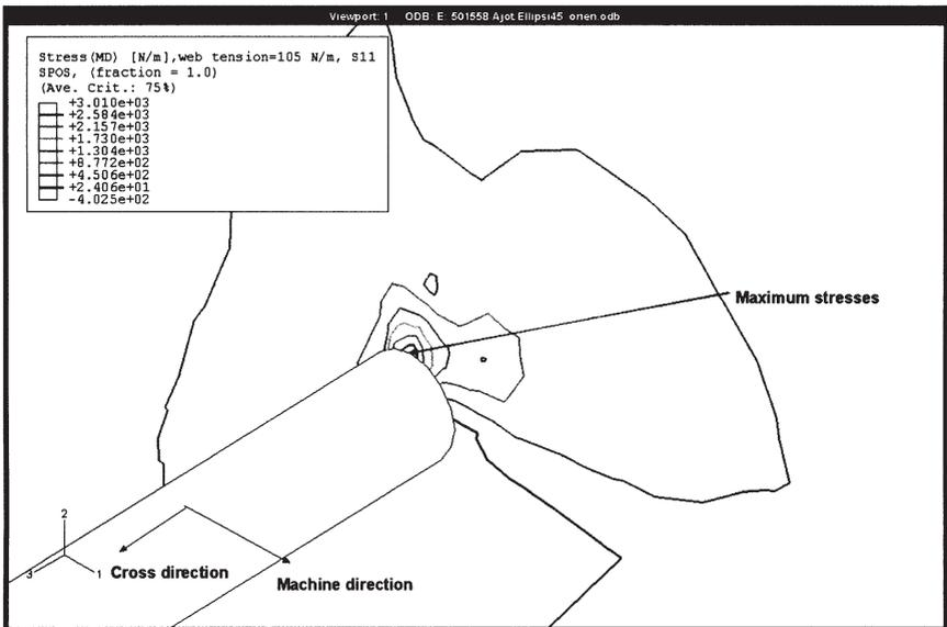
Figure 17 The dependency between web tension and maximum stress around a cut.
