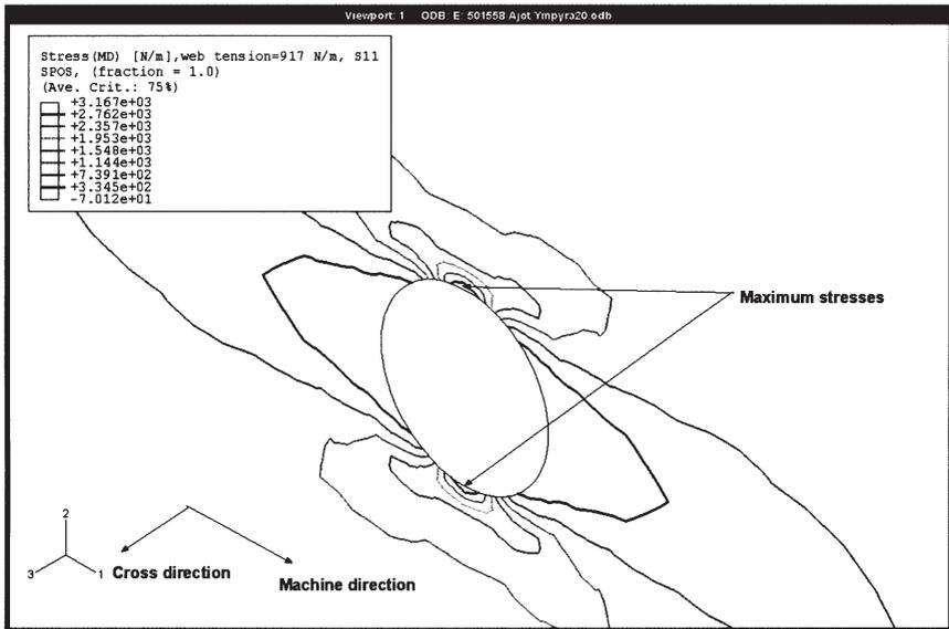
Figure 14 The dependency between web tension and maximum stress around a hole.
