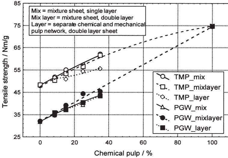
Figure 10 Tensile strength of single and double layered laboratory sheets. Chemical pulp was beaten in laboratory (Valley) to CSF 630 ml.
