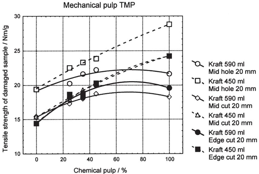
**Figure 4** The effect of defect shape and size on paper strength at various chemical pulp (bleached soft wood/pine kraft) addition levels. Mechanical pulp is TMP. Specimen width 50 mm.
