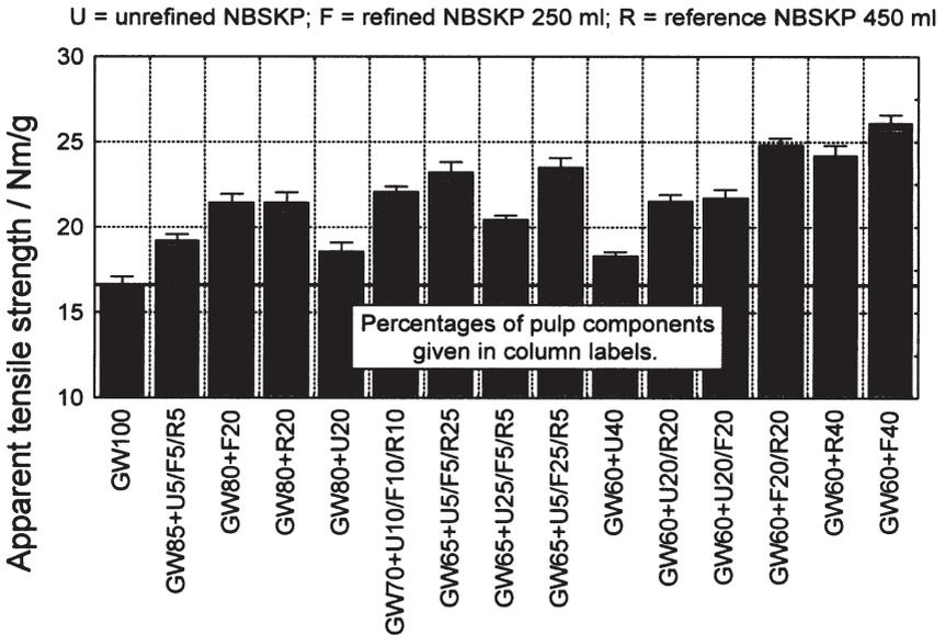
**Figure 9** The effect of chemical pulp refining and content on strength of damaged GW based paper. Values in column labels after each abbreviation of pulp name give the percentage shares of respective components.
