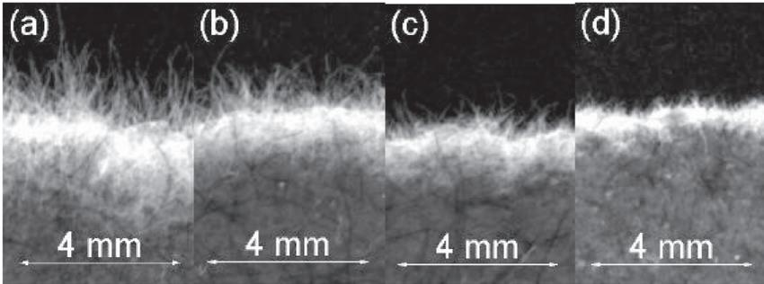
**Figure 9** Fracture lines in handsheets of bleached softwood kraft pulp. Fiber length, changed by cutting, increases from (a) to (d). Black area is scanner background (at top), white damage zone (middle) and dark gray undamaged paper (at bottom). The arithmetic mean fiber lengths (measured using Kajaani FS-100) were 0.7, 1.2, 1.9 and 2.8 mm and the length-weighted mean fiber lengths 0.8, 1.4, 2.2 and 3.1 mm, respectively [12].
