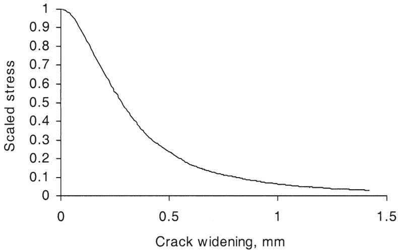
**Figure 3** A cohesive stress–crack widening curve. The stress values are renormalized by the maximum value.
