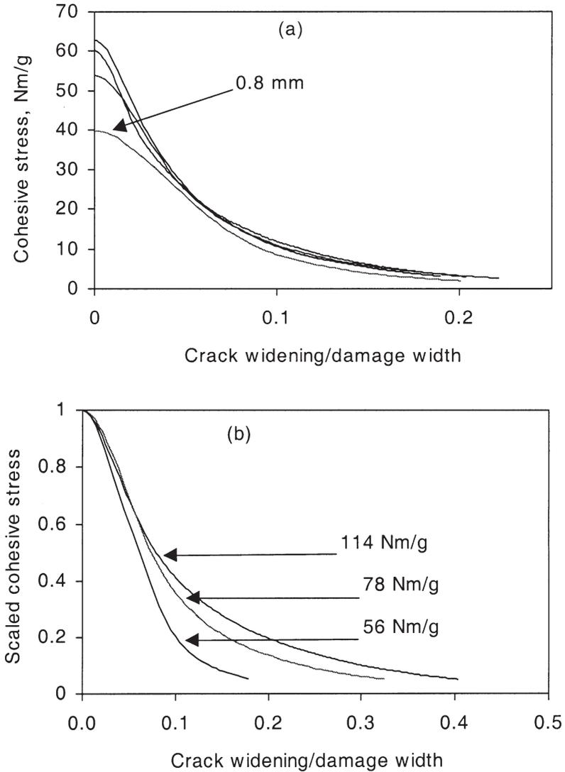
**Figure 4** Cohesive stress vs. crack widening values over damage width for samples with different fiber length (a) and different fiber strength (b). Fiber length was varied by cutting and reslushing handsheets and fiber strength was varied by HCl vapor exposure of handsheets. The original curves [7] were rescaled. Of different fiber lengths in (a), only the 0.8 mm case differs from the rest. In (b) the numbers indicate the zero span strength.
