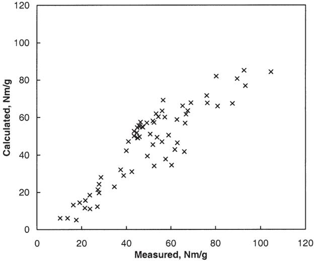
**Figure 7** Calculated (Equations 2 and 3) vs. measured values of the ordinary tensile index of handsheets containing various chemical pulps and their mixtures with mechanical pulps.
