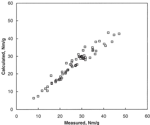
**Figure 6** Calculated (Equations 2 and 4) vs. measured values of the apparent tensile index of handsheets containing various chemical pulps and their mixtures with mechanical pulps.
