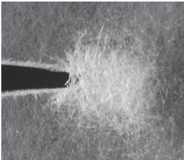
**Figure 2** Fracture process zone (FPZ, the white area) in a handsheet of pure softwood kraft. The crack is just about to start propagating to the right. The FPZ diameter is 3–4 mm.
