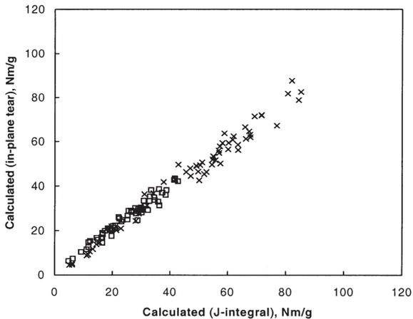
**Figure 8** Calculated values of the apparent (squares) and ordinary tensile index (crosses) of handsheets containing various chemical pulps and their mixtures with mechanical pulps. Comparison of in-plane tear test and J-integral method for measuring fracture energy.
