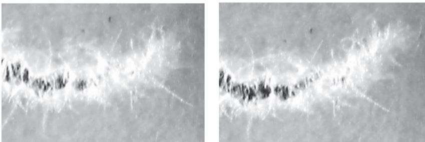
**Figure 1** Two successive images of the fracture process zone (FPZ) in a silicone impregnated handsheet of PGW plus 10% softwood kraft. The crack propagates from left to right. The images are taken against a black background that shows through the crack opening. The white color arises from broken inter-fiber bonds and fiber fractures that reflect light. The white fracture process zone is roughly 1 mm wide.
