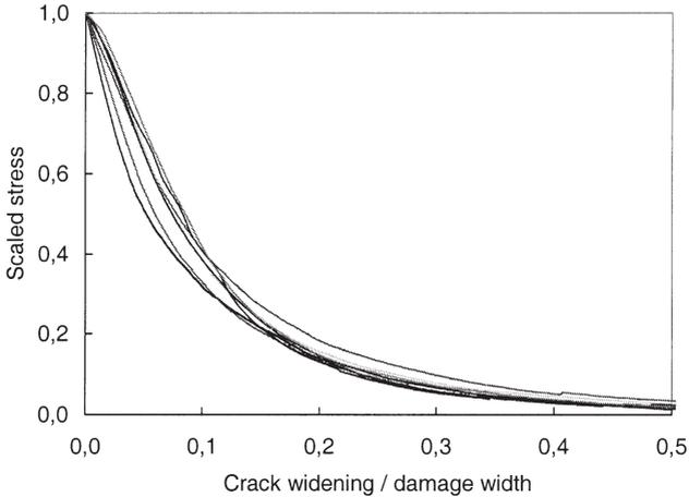
**Figure 5** Cohesive stress curves for mixtures of PGW and coarse spruce kraft. The mixing ratio has no systematic effect on the curves.
