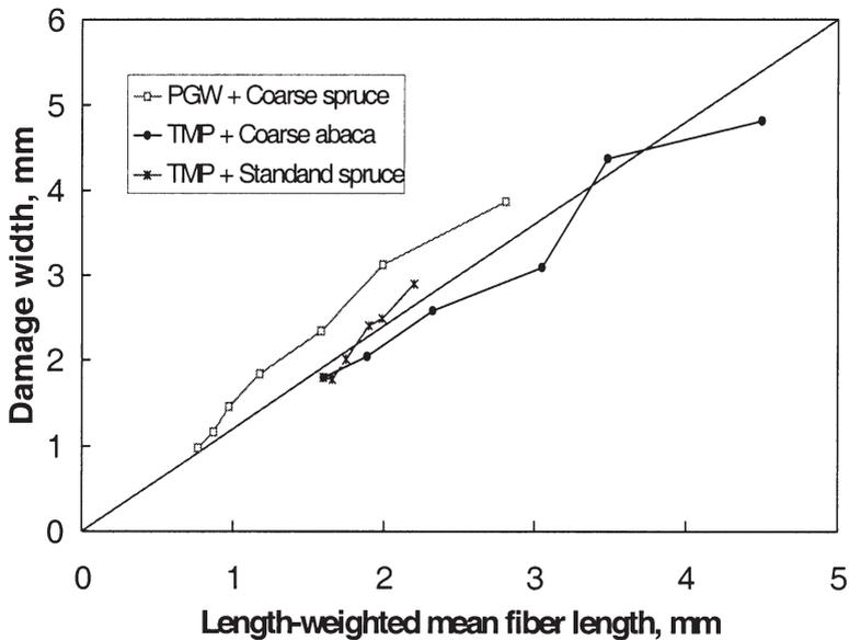
**Figure 10** Damage width against the length-weighted mean fiber length in mixtures of chemical and mechanical pulps. The fraction of chemical pulp ranges from 0 to 100% (from bottom left to top right). The straight line is only for illustration.
