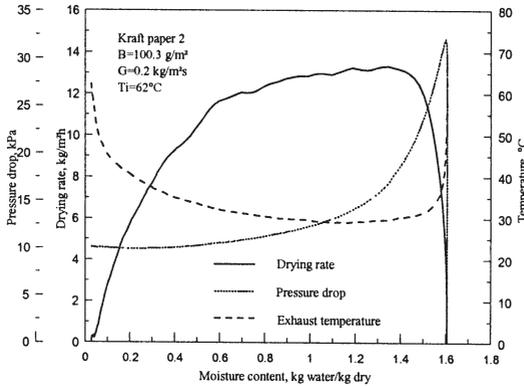
Figure 3 Through air drying for initial moisture content higher than FSP
