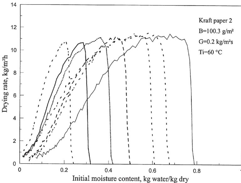
**Figure 12** Enhancement of through drying characteristics for initial moisture contents below FSP value
