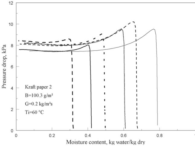
**Figure 14** Effect on through flow pressure drop for initial moisture contents below FSP value
