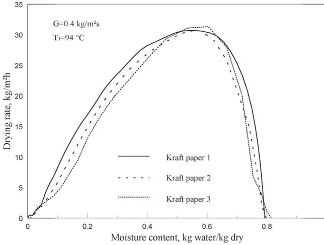
**Figure 8** Drying rate curves for 3 types of kraft paper;  $X_o = \text{FSP}$
