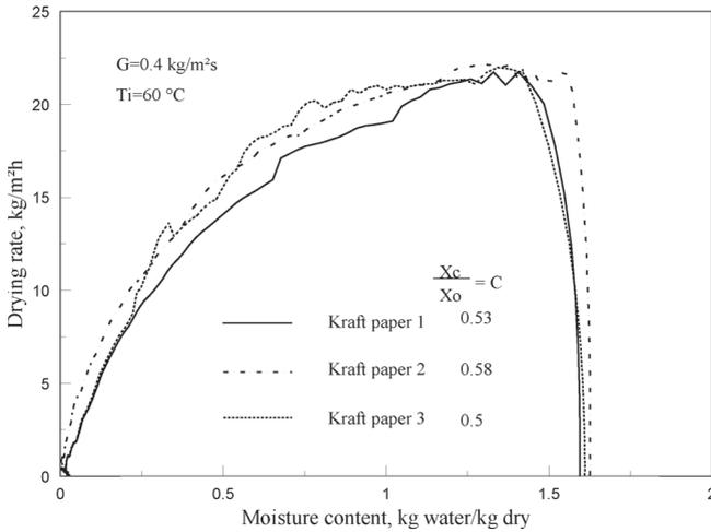
**Figure 7** Drying rate curves for 3 types of kraft paper:  $X_o > \text{FSP}$
