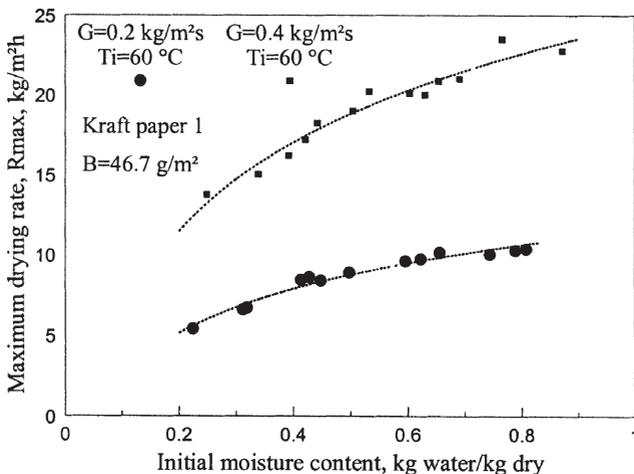
**Figure 17** Effect of initial moisture content on  $R_{\text{max}}$ : Kraft paper 1
