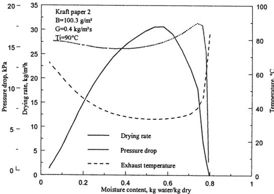
Figure 4 Through air drying for initial moisture content lower than FSP
