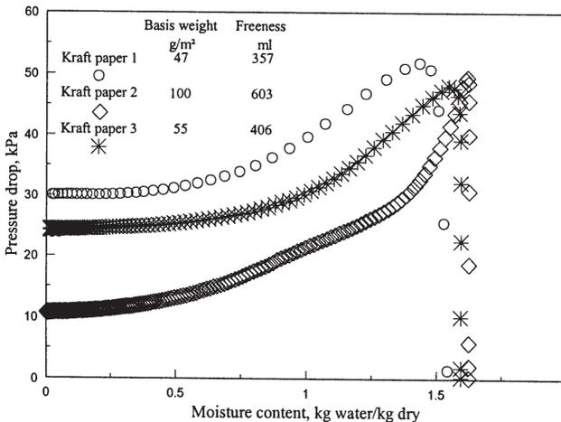
**Figure 5** Effect of moisture content on pressure drop for air flow through paper
