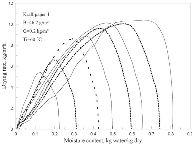
**Figure 15** Enhancement of through drying rate characteristics for initial moisture contents below FSP value: Kraft paper 1
