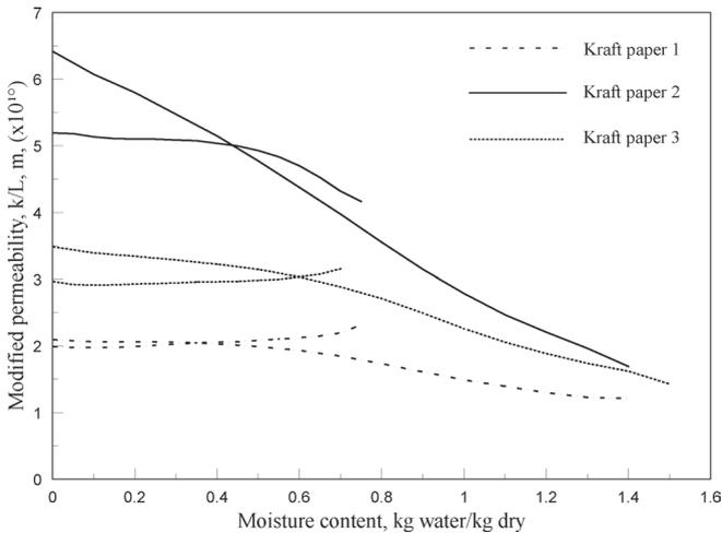
**Figure 6** Effect on modified permeability of kraft paper from initial moisture content of through drying
