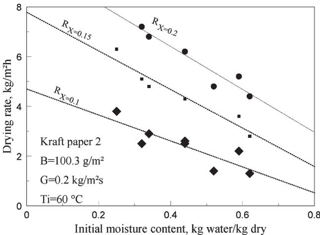
Figure 13 Enhancement of drying rate from reducing initial moisture content
