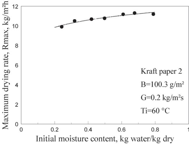
Figure 18 Effect of initial moisture content on  $R_{max}$ : Kraft paper 2
