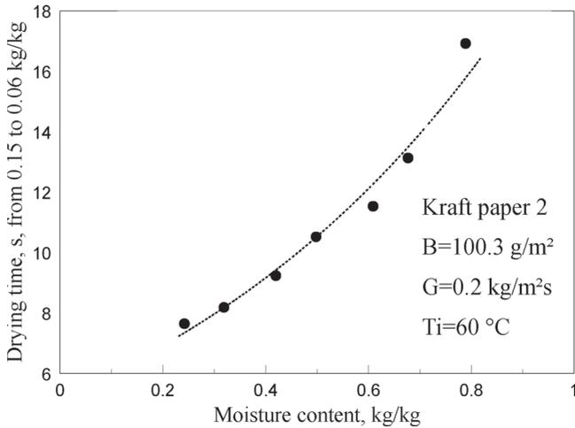
Figure 19 Reduction in drying time for initial moisture content below FSP value: Kraft paper 2
