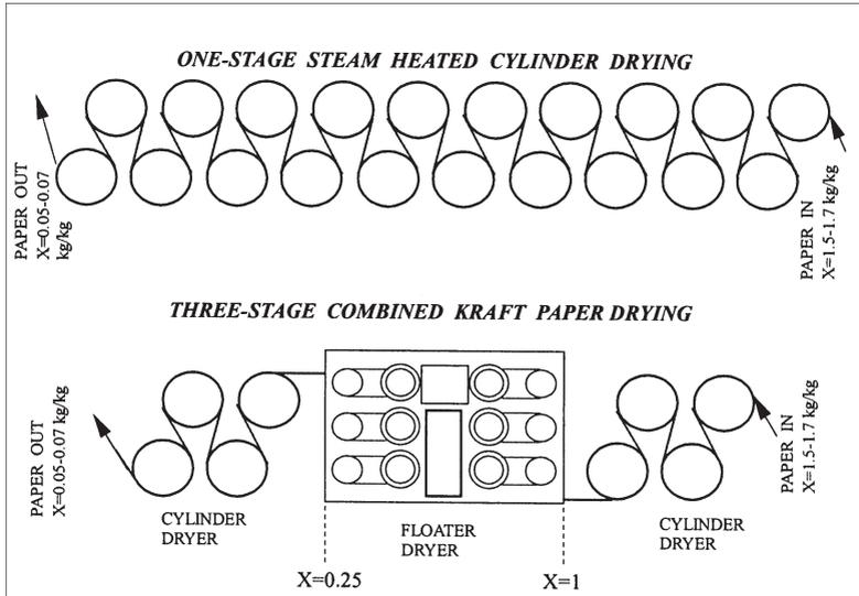
**Figure 1** Drying configurations for kraft paper
