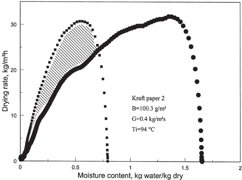
**Figure 11** Enhancement of through drying rate for a lower initial moisture content
