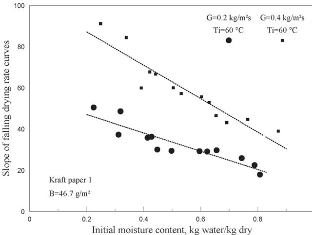
**Figure 16** Effect of initial moisture content on slope of falling rate drying curve: Kraft paper 1
