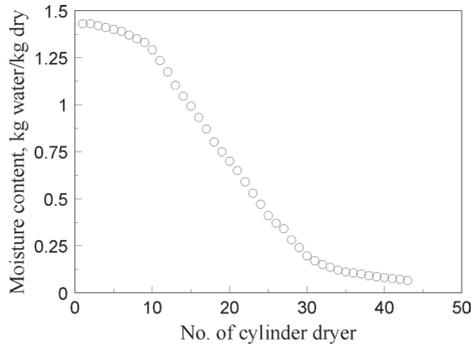
**Figure 2** Evolution of moisture content in cylinder drying
