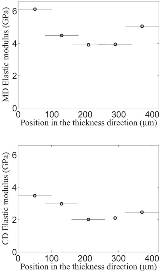
**Figure 14a,b** Experimental elastic moduli for layers of a board (circles), with horizontal lines showing the positions and thicknesses of the layers.
