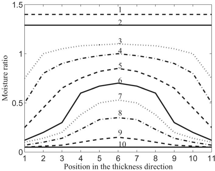
**Figure 7** Moisture history used in the simulations, with 3 minutes between the states shown in the graph, the states being numbered to be able to reference them later.
