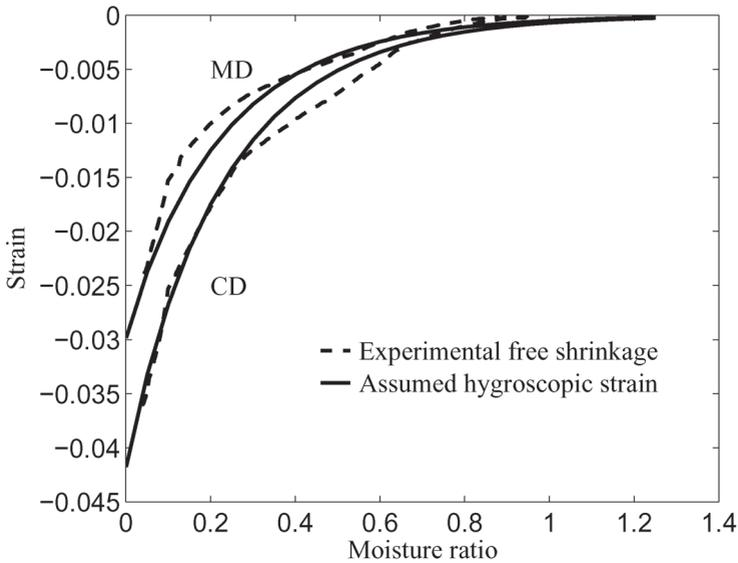
**Figure 1** Free shrinkage data and fitted curves.
