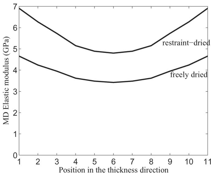
**Figure 13** MD elastic modulus as a function of position through the thickness, simulation results for restrained and free drying.
