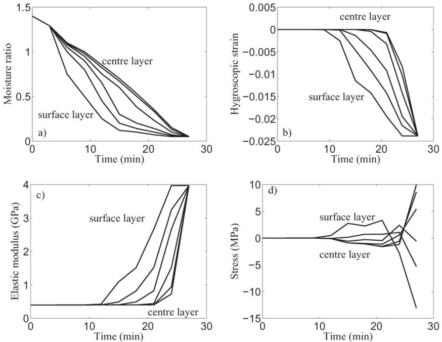
**Figure 8a,b,c,d** In a), moisture history for the different layers. In b), hygroscopic shrinkage history for the different layers. The surface layers dry and shrink first. In c), elastic stiffness development for the different layers. The surface layers stiffen first. In d), stress development at free drying for the different layers. The surface layers end up with the most compression.
