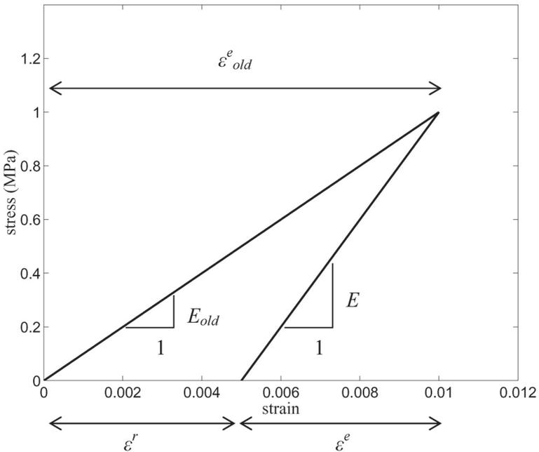
**Figure 3** Illustration of the inelastic strain, which is the strain that remains when the stress (and the elastic strain) has returned to zero in the example.
