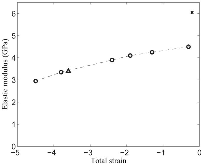
**Figure 16** Elastic modulus simulation data as a function of total strain (%) after drying. The circles connected by a dashed line are the CD results for varying applied strain in that direction when the strain in the MD was restrained. The MD results for the same cases are shown by the crosses (all on top of each other). The triangle is the CD result for free drying in both directions and indeed falls practically on the dashed curve.
