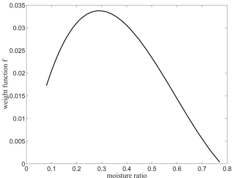
**Figure 6** Weight function for the influence of stresses on elastic moduli (Equation (12)).
