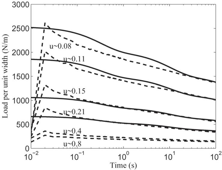
**Figure 4a** Stress relaxation data at various moisture ratios and 1.0% applied strain (dashed), and modelling of this relaxation (solid curves) for a few of the tests once the constant strain has been applied, using the same set of time constants for all the solid curves.
