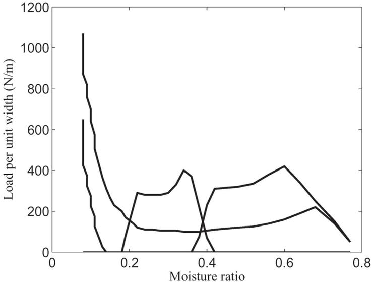
**Figure 5** Uniaxial load histories during drying for four different tests, as support to the proposed model of the effect of drying restraints on stiffness (Equations (10–12)). The corresponding stiffnesses are given in Table 1.
