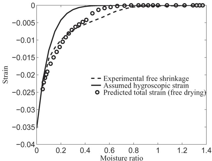
**Figure 10** Free shrinkage in the MD as a function of moisture ratio.
