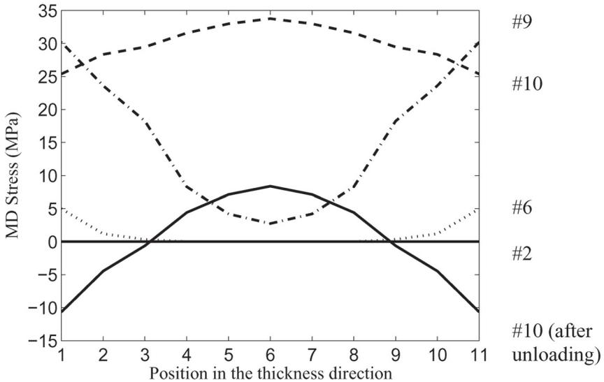
**Figure 12** Distribution of MD stress through the thickness for different times during restrained drying. The number of the moisture profile in Figure 7 that the results correspond to is shown at the right end of the curves.
