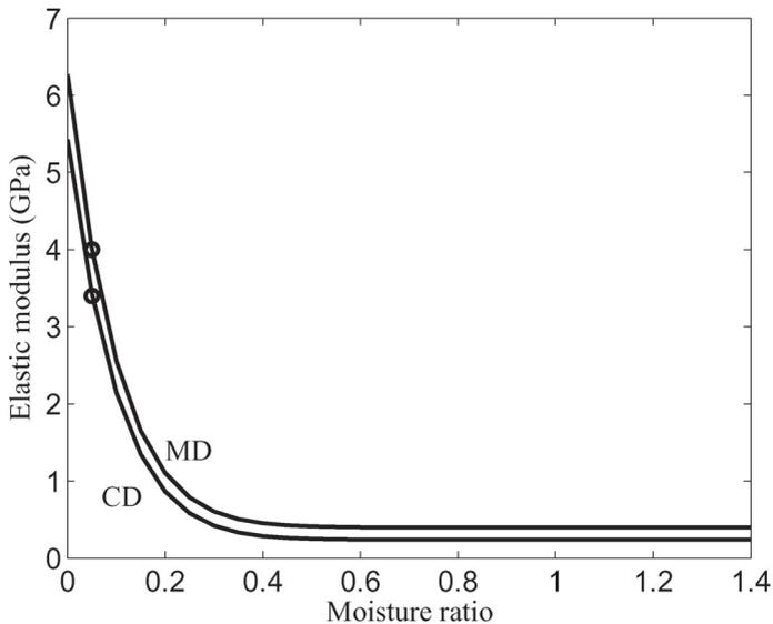
**Figure 2** Stiffness development at free drying, with circles representing the experimental dry stiffness data of the studied freely dried board.
