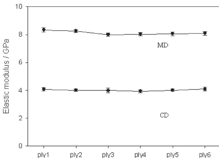
**Figure 15** Experimental elastic moduli for plies of a board couched from papers formed individually and couched before drying, to avoid structural variation.
