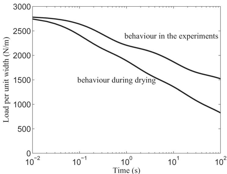
**Figure 4b** Simulations of relaxation tests. The upper curve is obtained with the time constants in Figure 4a, the lower curve shows the same test with the time constants used in the present drying simulations.
