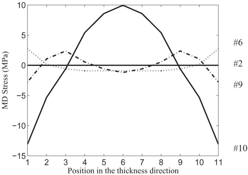
**Figure 11** Distribution of MD stress through the thickness for different times during free drying. The number of the moisture profile in Figure 7 that the results correspond to is shown at the right end of the curves.
