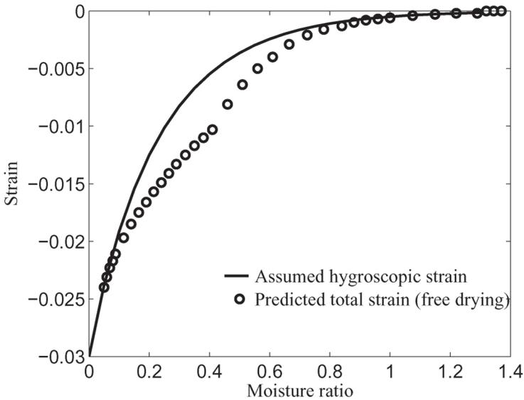
**Figure 9** Free shrinkage in the MD as a function of moisture ratio.
