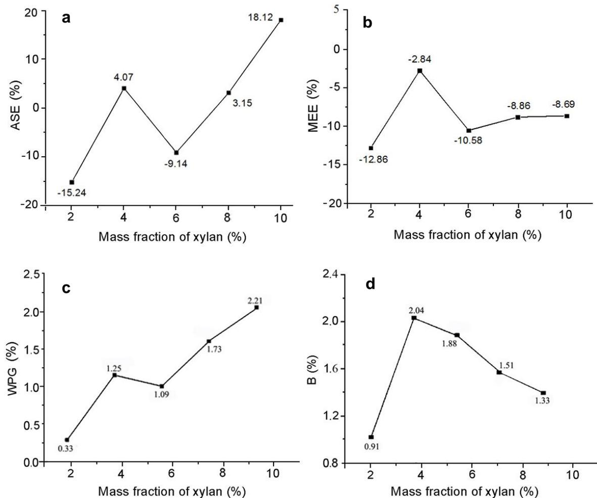
**Fig. 3.** (a) ASE, (b) MEE, (c) WPG, and (d) B of bamboo specimens modified by different mass fractions of xylan
