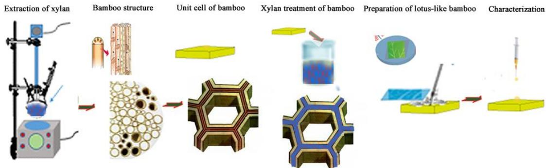
**Fig. 2.** Treatment for dimensional stability of lotus leaf-like bamboo by xylan
