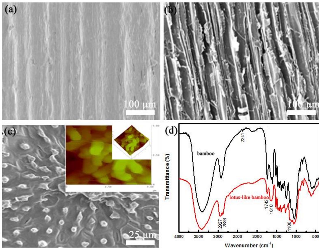
**Fig. 4.** The SEM images and FTIR of the samples: (a) bamboo surface, (b) xylan-treated bamboo surface, (c) modified lotus leaf-like bamboo surface, and (d) FTIR spectra
