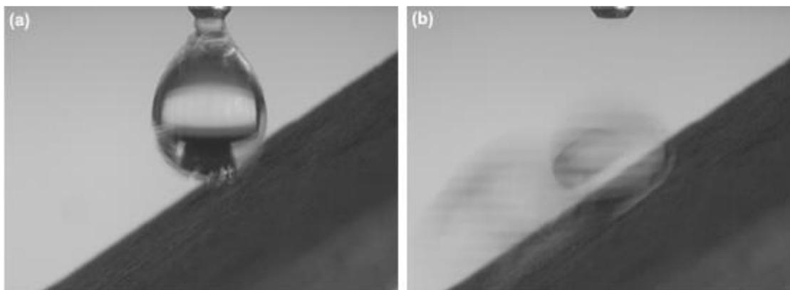
**Fig. 6.** WAC images of samples with (a) and (b) a rolling process of water on modified lotus leaf-like bamboo surface
