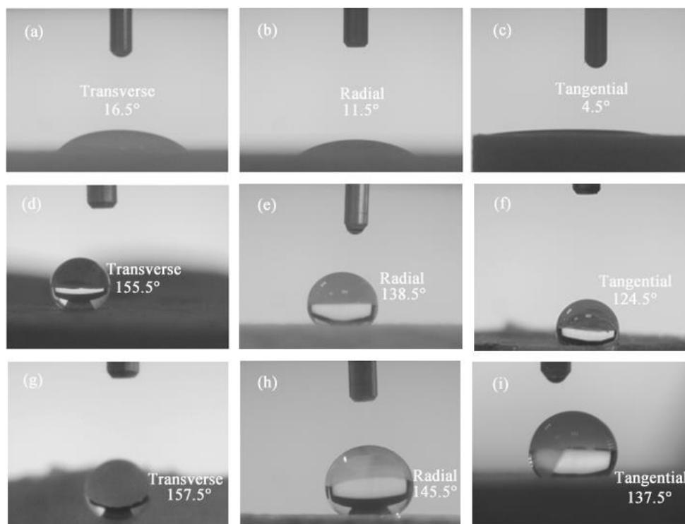
**Fig. 5.** The water contact angles (WCAs) of the different sections of (a through c) bamboo, (d through f) unmodified lotus leaf-like bamboo, and (g through i) modified lotus leaf-like bamboo
