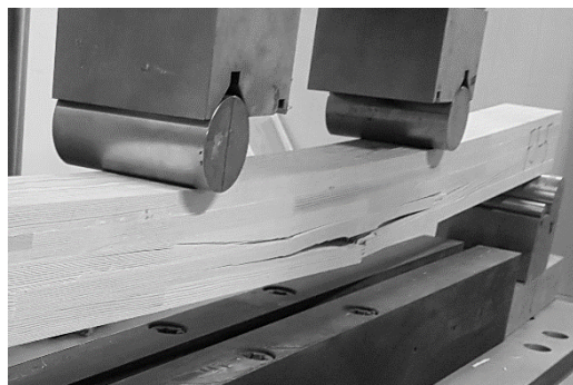
(a) Tension failure
