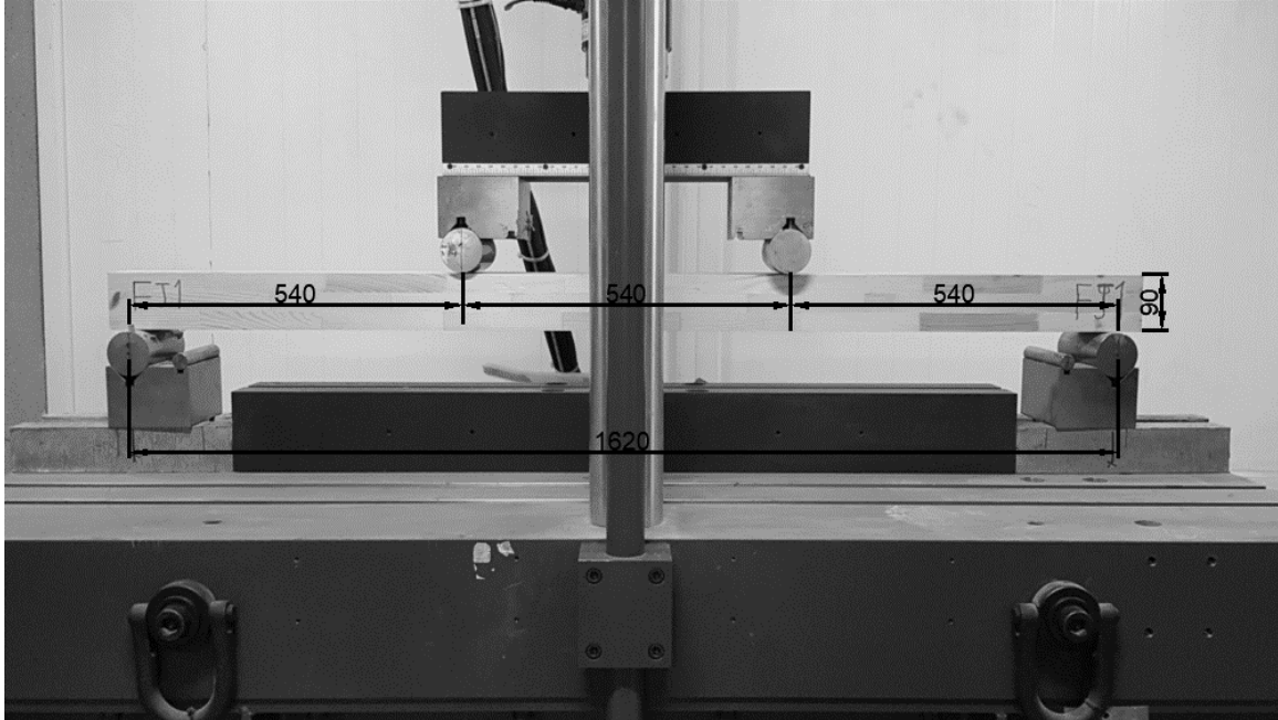
Fig. 5. The four-point bending test arrangement of the specimens
