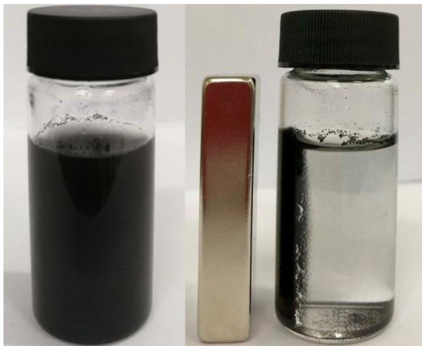
Fig. S2. Attraction of catalyst by an external magnetic field
