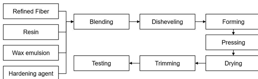
**Fig. 1.** The wood-fiber insulation board manufacturing process
