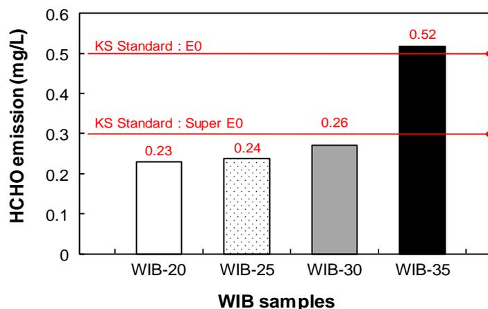
**Fig. 4.** The HCHO emission of the WIB samples with varying resin content (20, 25, 30, and 35%)
