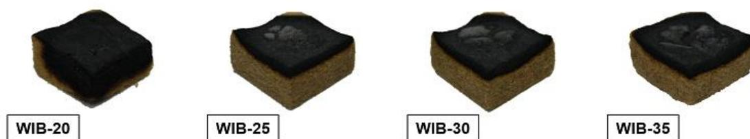
**Fig. 5.** Specimen shapes of the WIB samples with varying resin content (20, 25, 30, and 35%) after the perpendicular flame test
