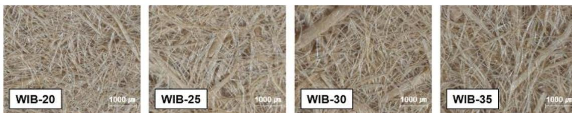
**Fig. 2.** Stereo microscope images (25x) of the WIB samples with varying resin content (20, 25, 30, and 35%).
