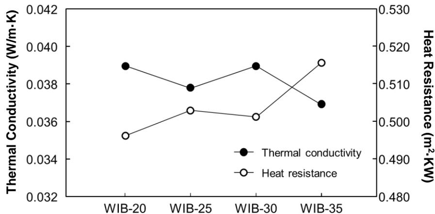
**Fig. 3.** The thermal conductivity and heat resistance of the WIB samples with varying resin content (20, 25, 30, and 35%)
