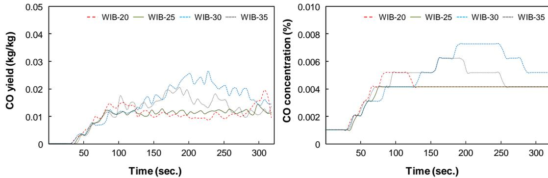
**Fig. 7.** CO yield (left) and concentration (right) of the WIB samples with varying resin content (20, 25, 30, and 35%)
