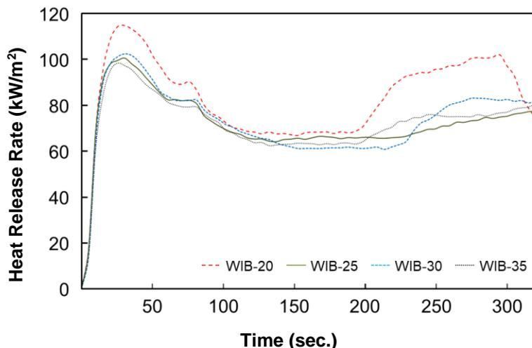
**Fig. 6.** The HHR curves of the WIB samples with varying resin content (20, 25, 30, and 35%).
