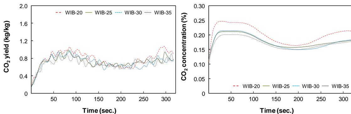
**Fig. 8.** CO<sub>2</sub> yield (left) and concentration (right) of the WIB samples with varying resin content (20, 25, 30, and 35%)
