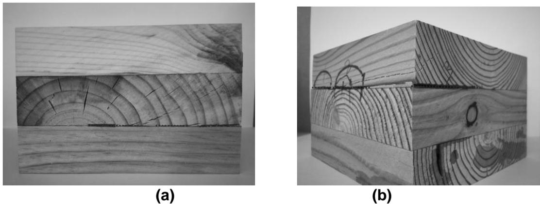
Fig. 7. Typical delamination seen in CLT specimens: (a): side view, (b): isometric view
