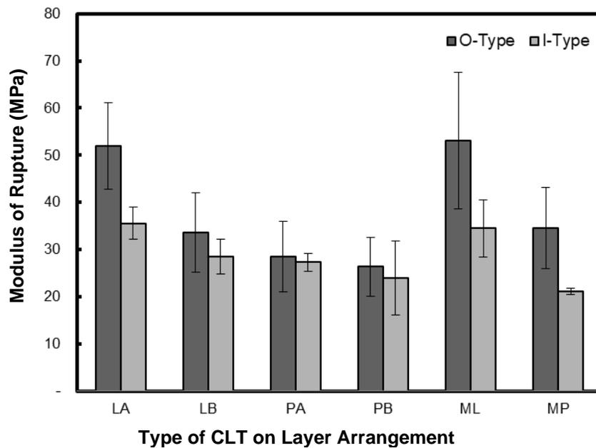
Fig. 9. Comparison of bending MOR by arrangements of CLT layers
