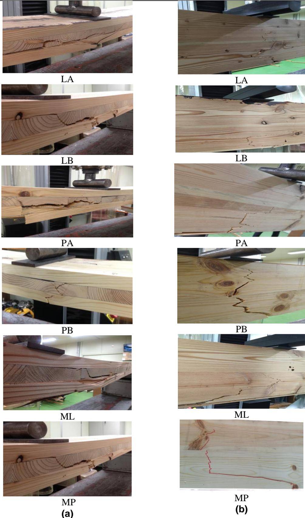
Fig. 11. Typical bending failures by loading direction (a: O-type, and b: I-type)
