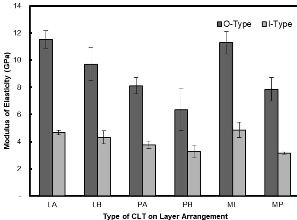
Fig. 10. Comparison of bending MOE by arrangement of CLT
