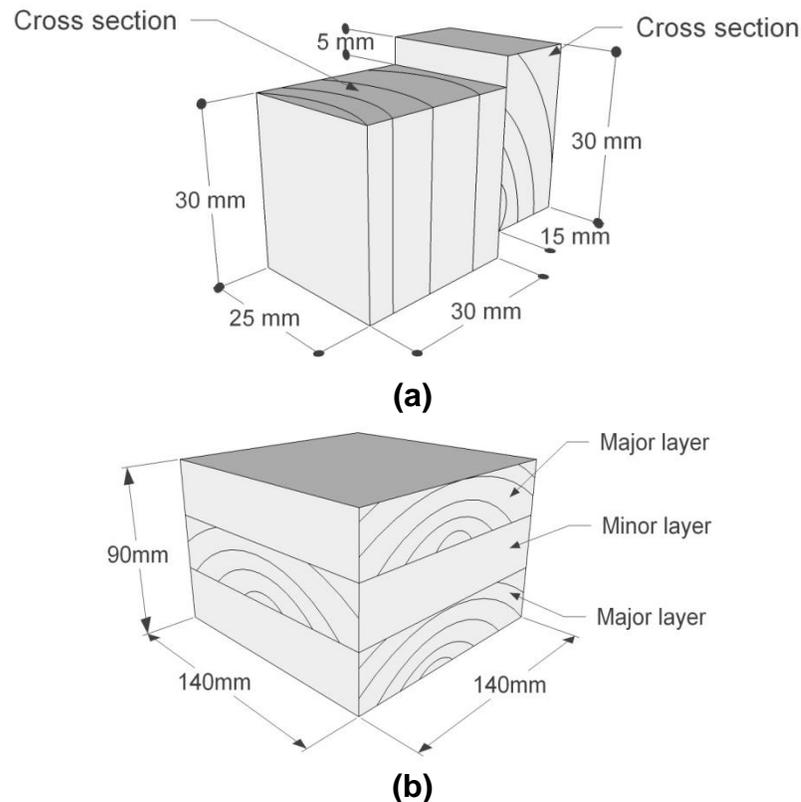
**Fig. 4.** Schematics of bonding test specimens: (a): Block shear and (b): Soaking delamination
