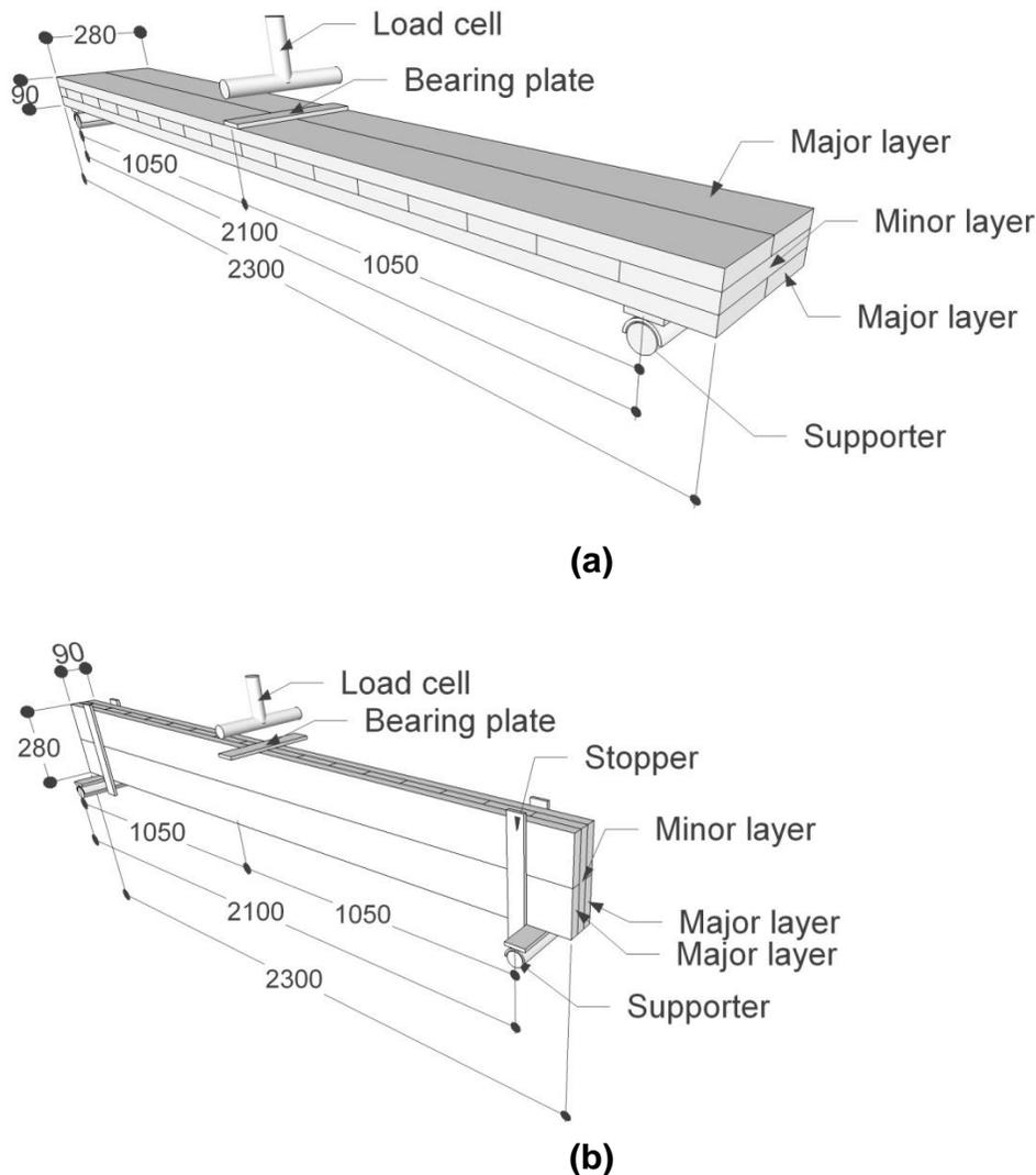
**Fig. 5.** Schematics for bending test based on the loading direction: (a): O-type, (b): I-type, and unit: mm
