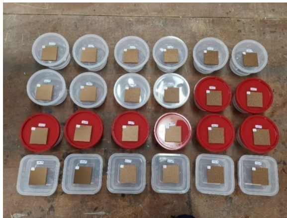
Fig. 3. Preparation of sample for thickness swelling and water absorption test
