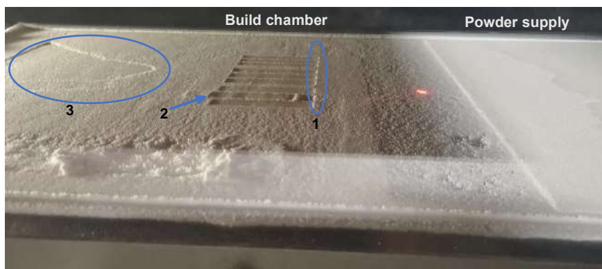
Fig. 1. Laser sintering of neat PLA: (1) Warping near the parts' edge; (2) displacement caused by the deformation; (3) lack of feedstock caused by the shrinkage of PLA
