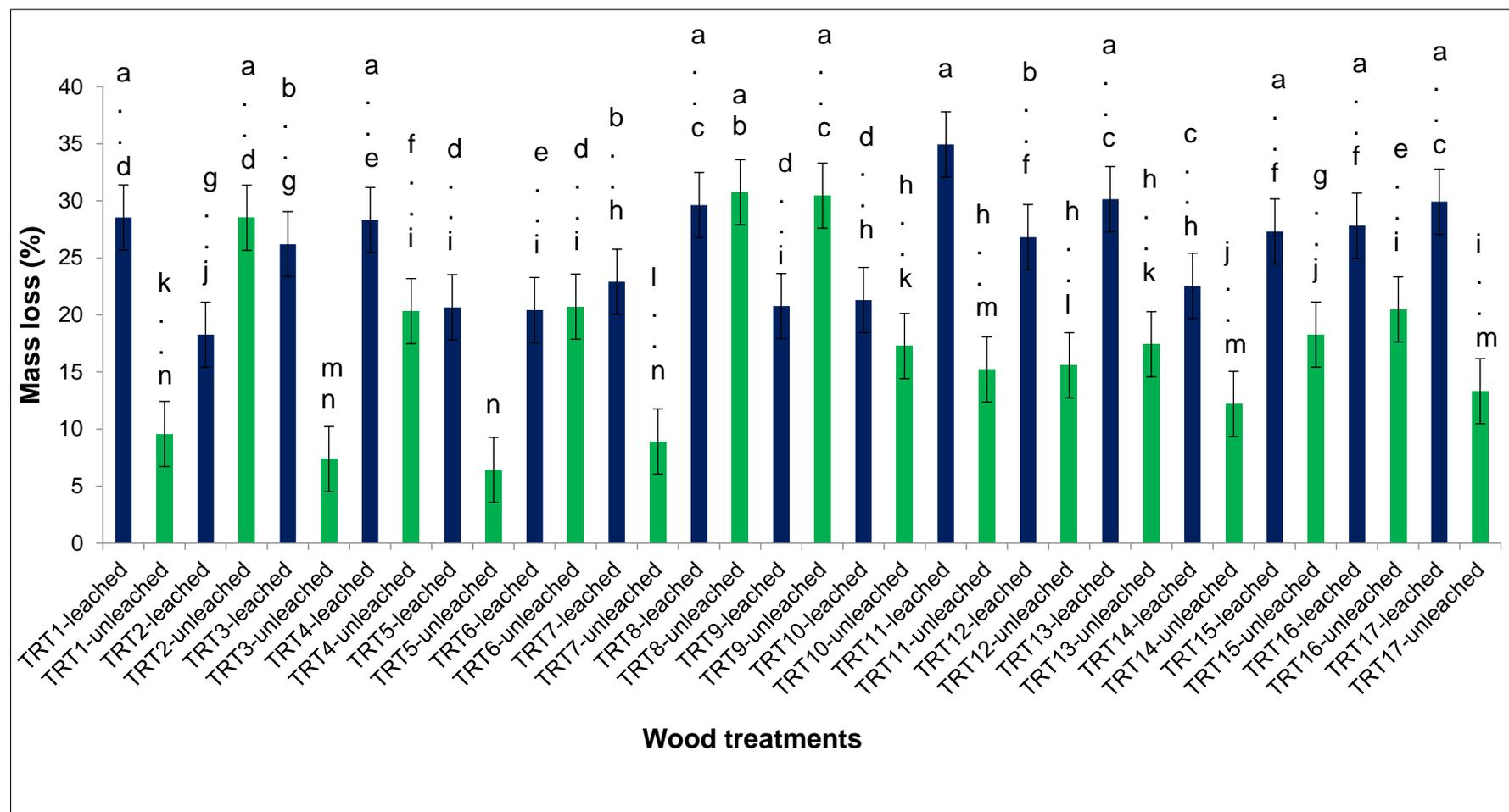
**Fig. 1.** The mass loss (ML) results of the 17 brown rot fungi (*Gloeophyllum trabeum*) wood treatments (leached and unleached samples). \*All treatments from 1 to 17 (TRT1 to TRT 17) were described in Table 1. In addition, treatments 1 to 17 were also tested in leached and unleached conditions which is illustrated in this figure.
