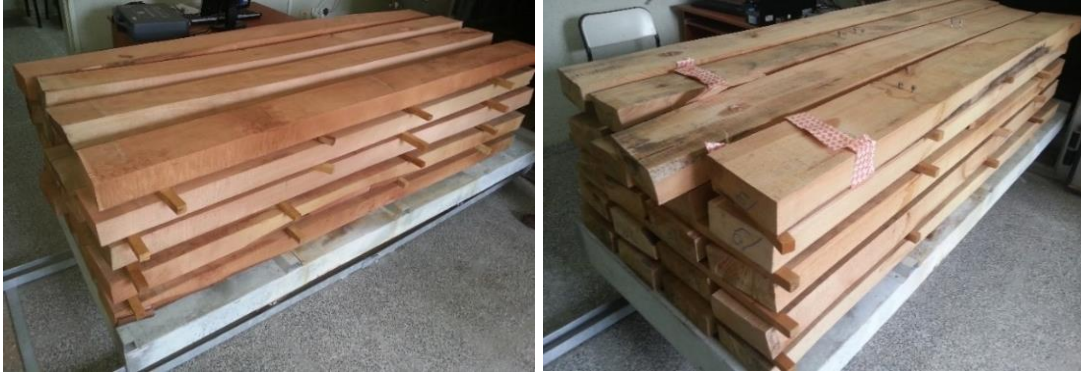
Fig. 4. Drying results for oriental beech: (Left) protective; (Right) severe drying
