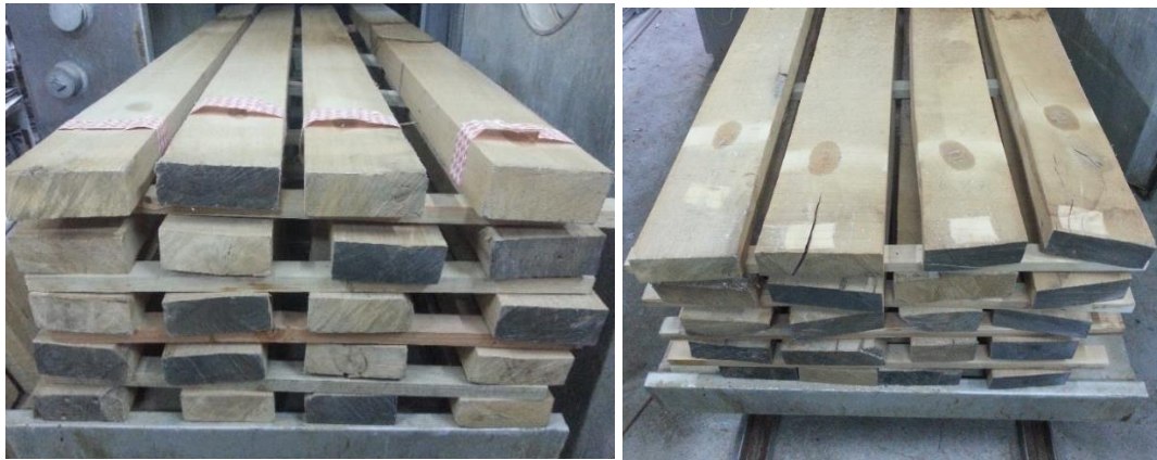
Fig. 5. Drying results for sessile oak: (Left) protective; (Right) severe drying
