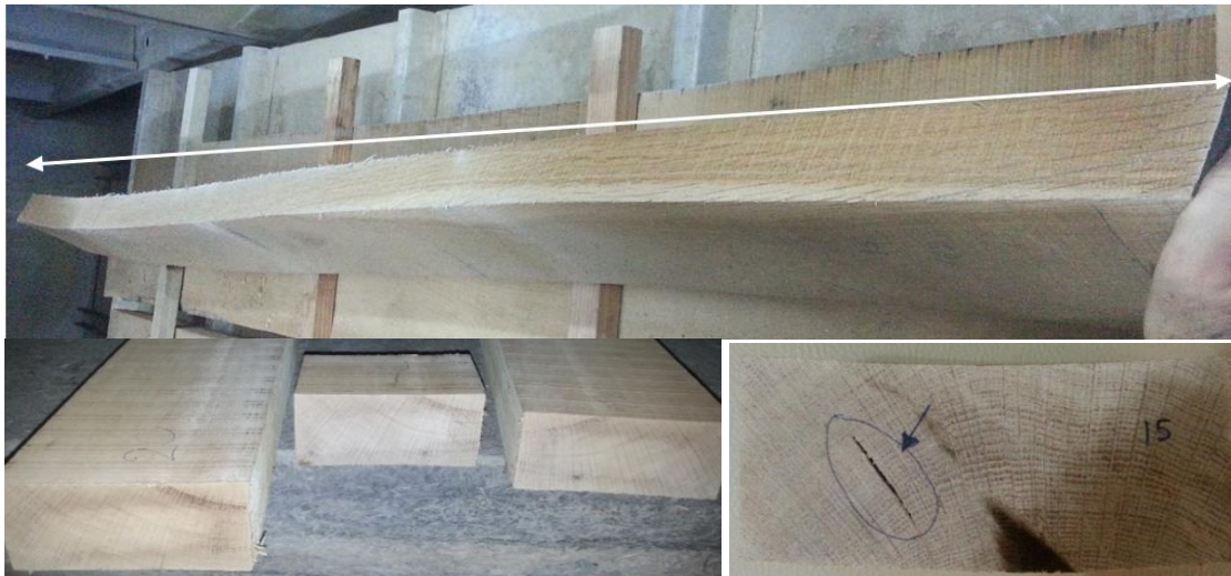
Fig. 6. Quality problems (distortion, case hardening, and honeycombing) in severe drying of sessile oak
