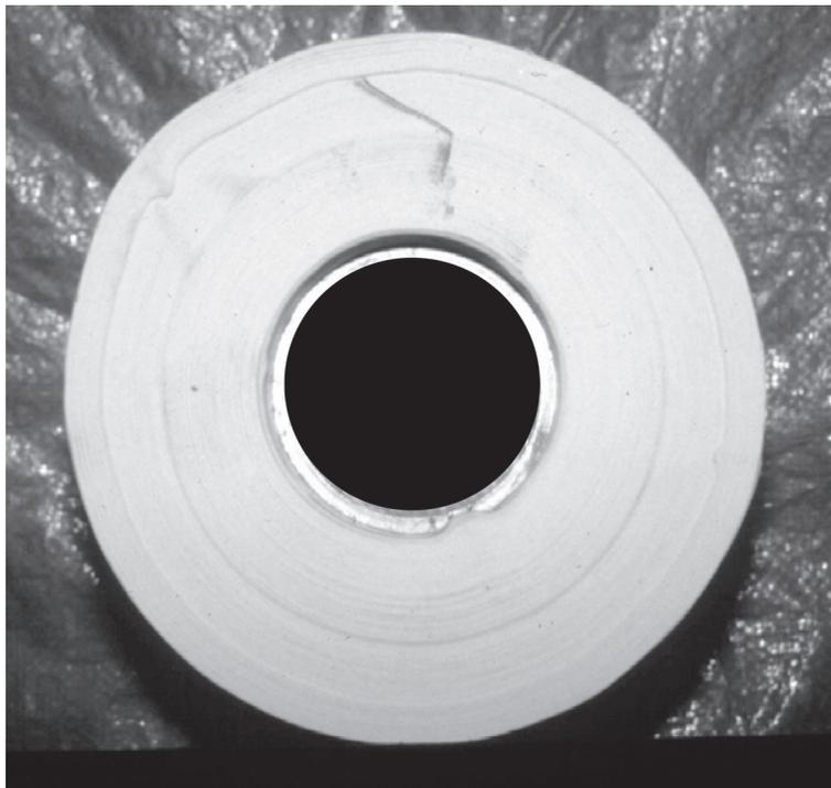
**Figure 44** Newsprint Roll Center Wound at the Winding Tension Profile shown in Figure 40.
