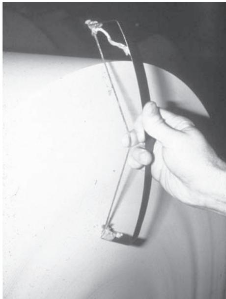
**Figure 62** Striking a “J-Line” to Investigate in Roll Slippage.
