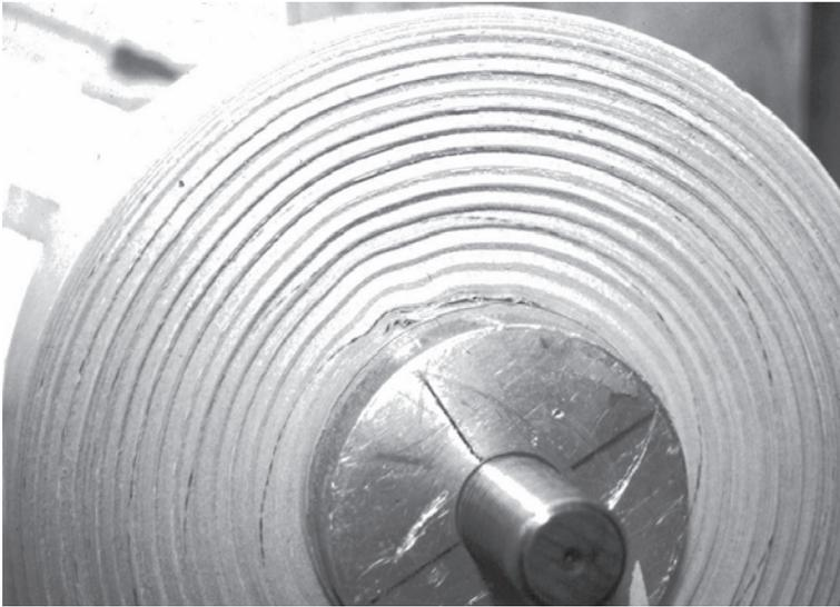
**Figure 45** Example of a Wound Roll Subjected to Inertial Torques in Excess of the Torque Capacity. Note the Spiral of the J-Line, which was a Radial Line Prior to Deceleration, and the Crepe Wrinkles near the Core.
