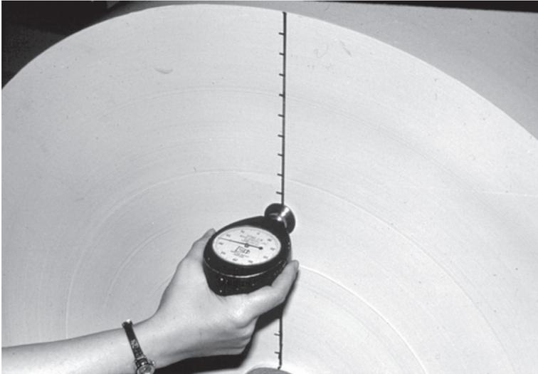
**Figure 59** The Smith Needle in an Evaluation of In-Roll Pressure.
