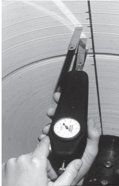
**Figure 58** Pull Tab Measurements of Roll Pressure.
