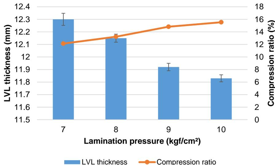
Fig. 2. Compression ratio and final thickness of rubberwood LVL with 7, 8, 9, and 10 kgf/cm<sup>2</sup>
