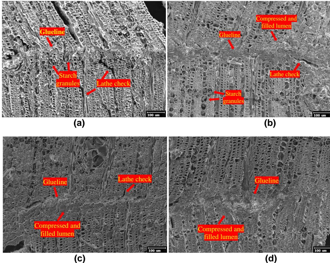
**Fig. 4.** Rubberwood LVL showing the glueline observed using SEM; LVL hot pressed at (a) 7 kgf/cm<sup>2</sup>; (b) 8 kgf/cm<sup>2</sup>; (c) 9 kgf/cm<sup>2</sup>; and (d) 10 kgf/cm<sup>2</sup> with 200x magnification
