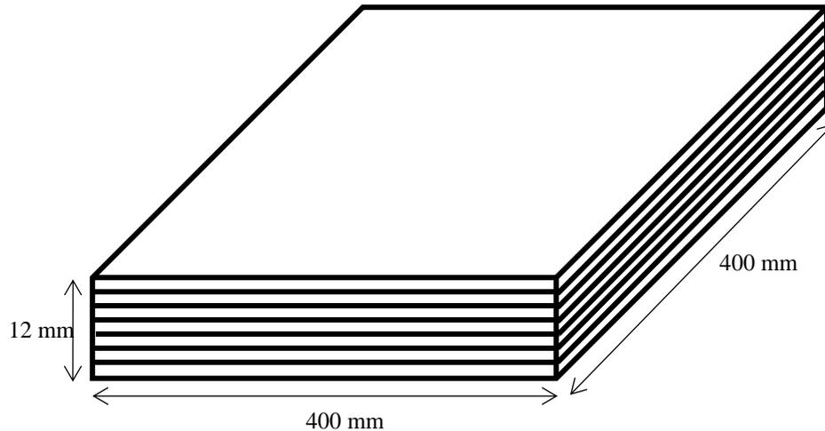
**Fig. 1.** The LVL with 12 mm thickness comprised of 7 ply of 2-mm-thick veneer
