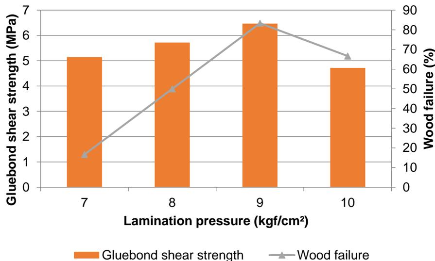
Fig. 3. Gluebond shear strength for rubberwood LVL pressed with 7, 8, 9, and 10 kgf/cm<sup>2</sup>
