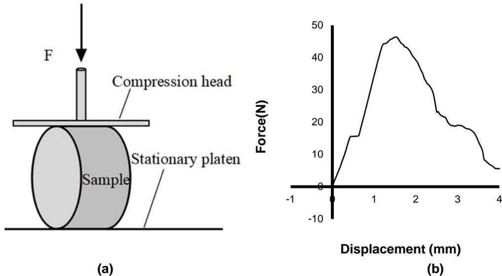
**Fig. 2.** Crushing resistance testing. (a) Loading direction; (b) curve of force with displacement
