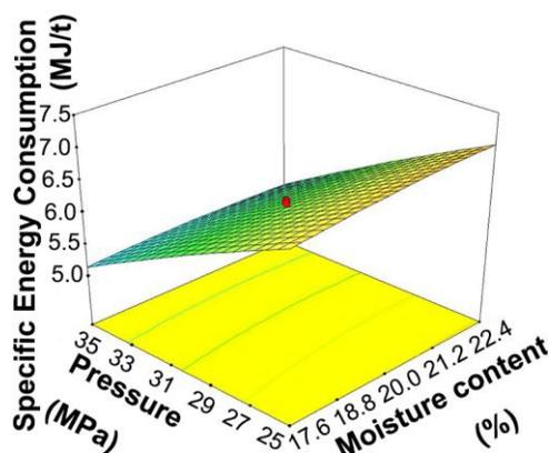
**Fig. 5.** Response surface plot representing effect of pressure and moisture content on specific energy consumption of briquetting (other factor is constant at zero levels)
