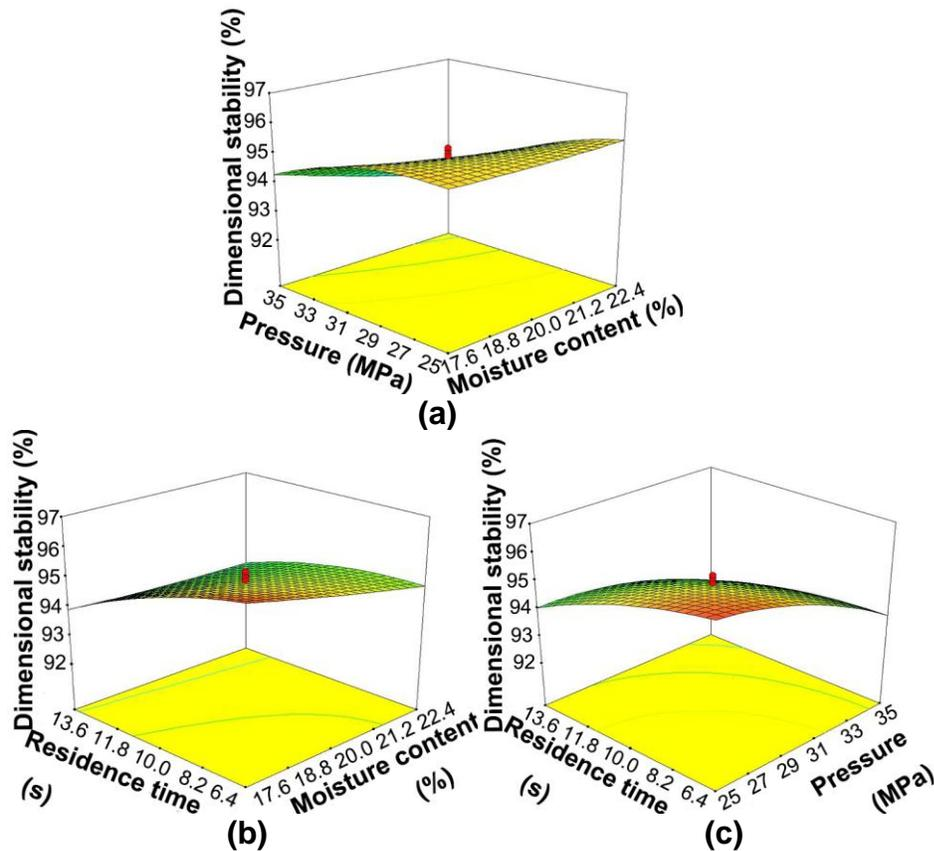
**Fig. 4.** Response surface plot for dimensional stability; other factors are constant at zero levels. The interactions between (a) moisture and pressure, (b) moisture and residence time and (c) pressure and residence time
