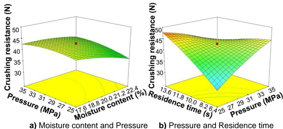
**Fig. 3.** Response surface plot representing effect of pressure and residence time on crushing resistance of biochar briquette (other factor is constant at zero levels). The interactions between (a) moisture and pressure; (b) pressure and residence time
