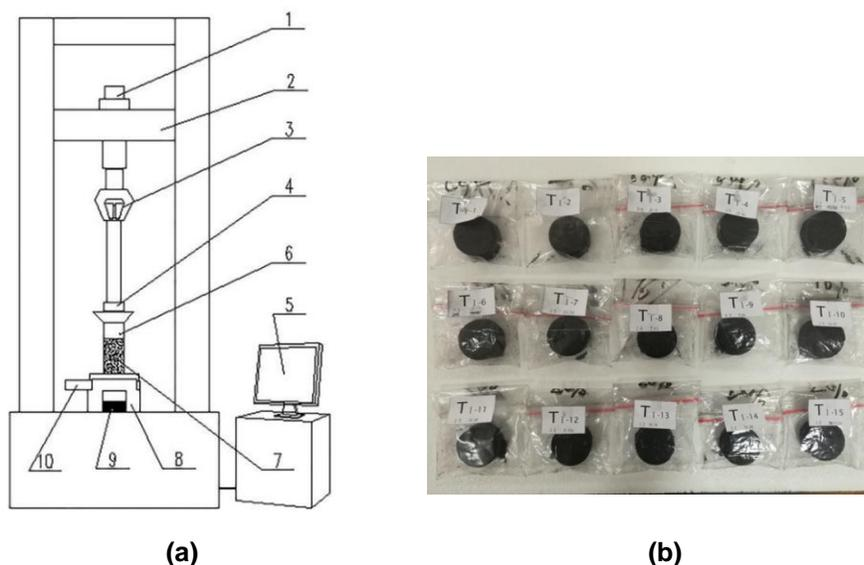
**Fig. 1.** Experimental system for biochar densification; (a) the experimental system: (1) sensor, (2) beam, (3) fixture, (4) compression head (5) computer, (6) cartridge, (7) biochar, (8) support, (9) biochar briquette, (10) sliding gate; (b) the formed biochar briquettes.
