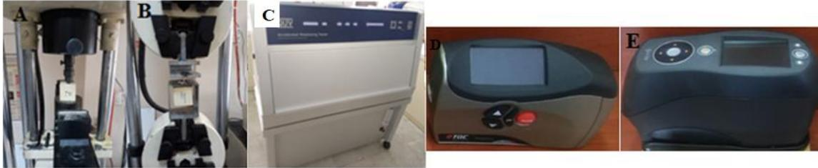
**Fig. 1.** Instruments used for different property measurement: (A) Janka hardness, (B) screw withdrawal resistance, (C) QUV weathering tester, (D) gloss meter, and (E) spectrophotometer
